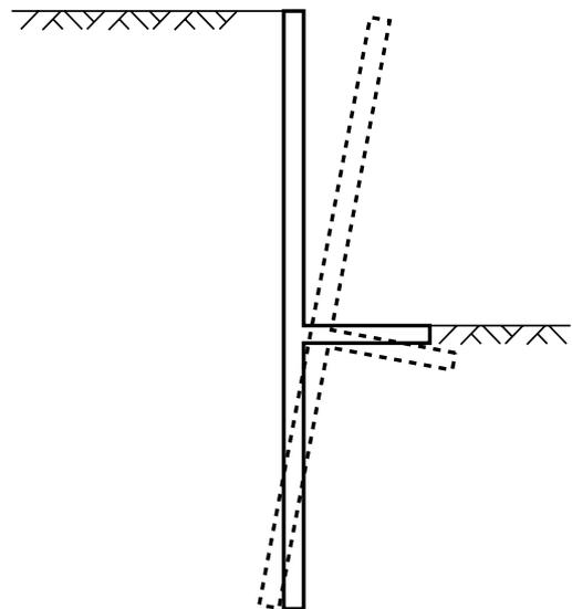
(d) Forward rotation about a point between the base and wall toe
