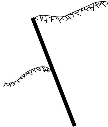
(b) Failure by forward rotation, if no ties present (cantilever)
