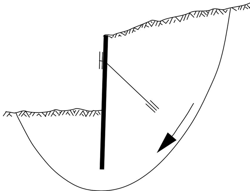
(c) Rotation failure of the mass of soil in which the structure is embedded
