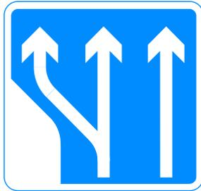
Fig. 9 Carriageway widens on Left (Lane addition other than at Junctions)
