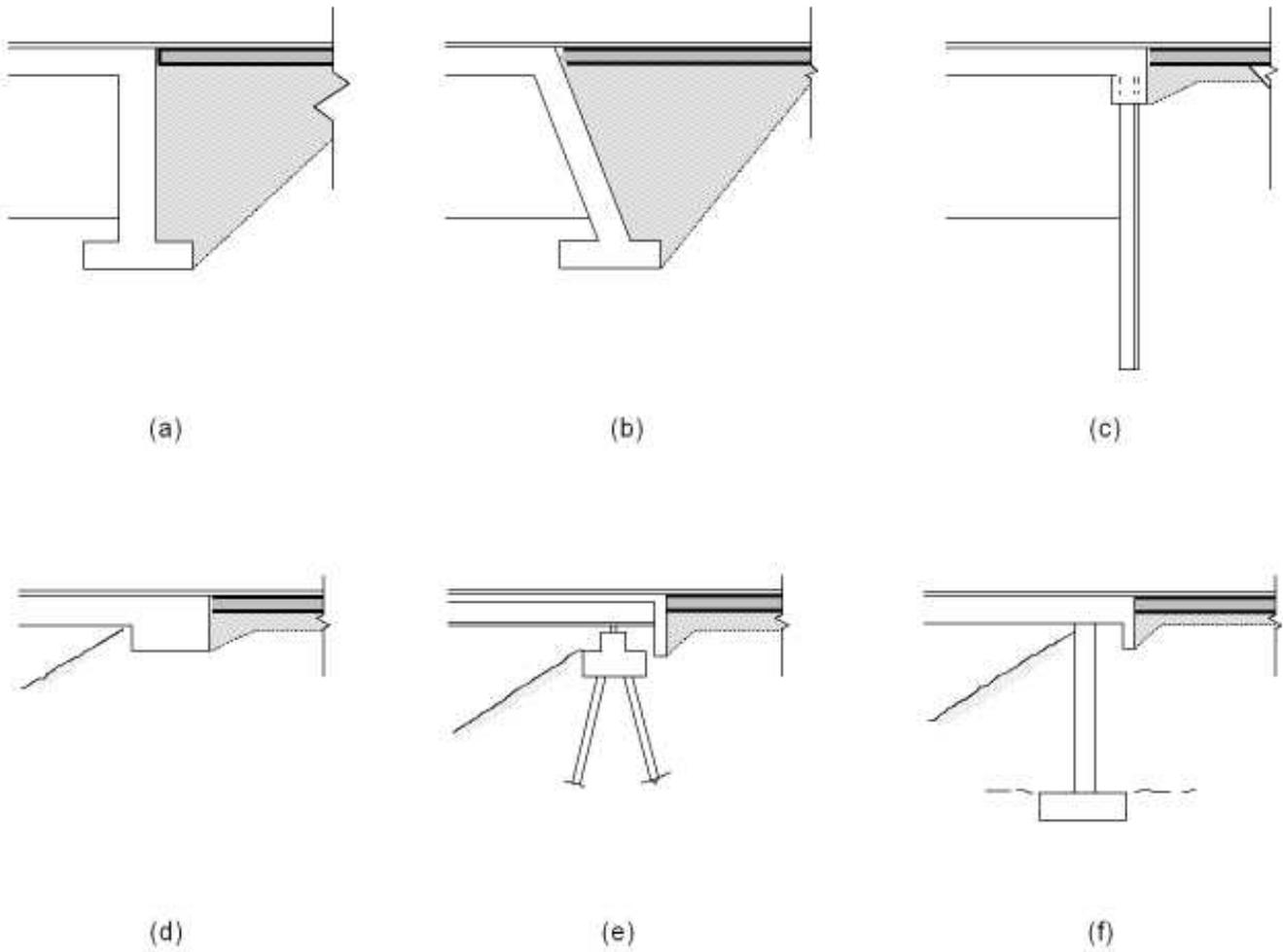
**Figure 2.1 Types of Integral Abutments**
