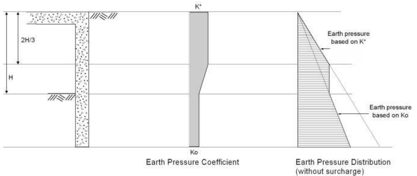
Figure 3.2 Earth Pressure Distribution for Full height Embedded Wall Abutments
