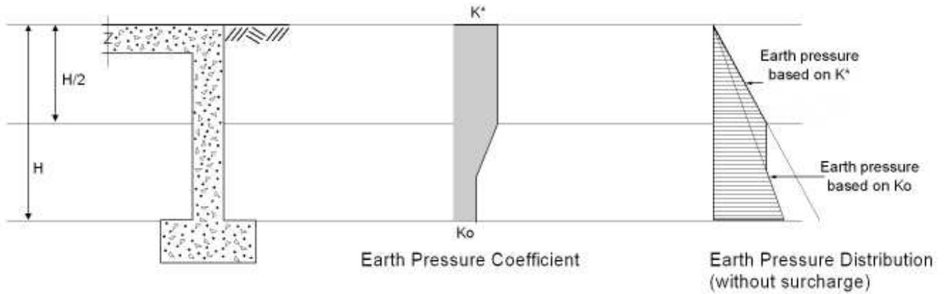
Figure 3.1 Earth Pressure Distribution for Frame Abutment
