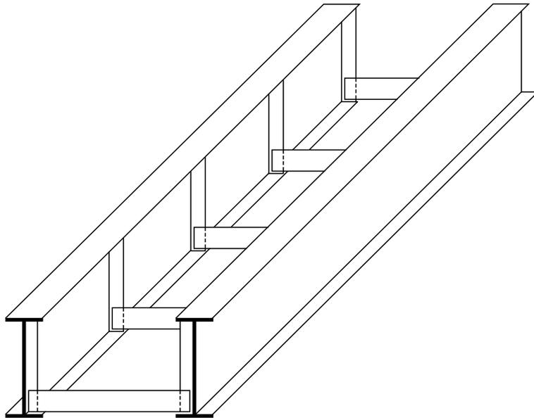
Figure 2 (a) Half through type bridge restrained by U-frame
