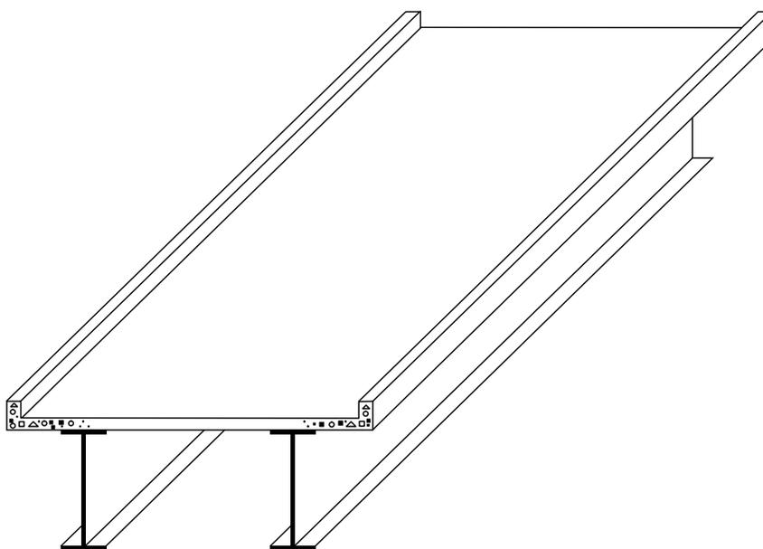
Figure 1 (b) Compression flange restrained by the deck
