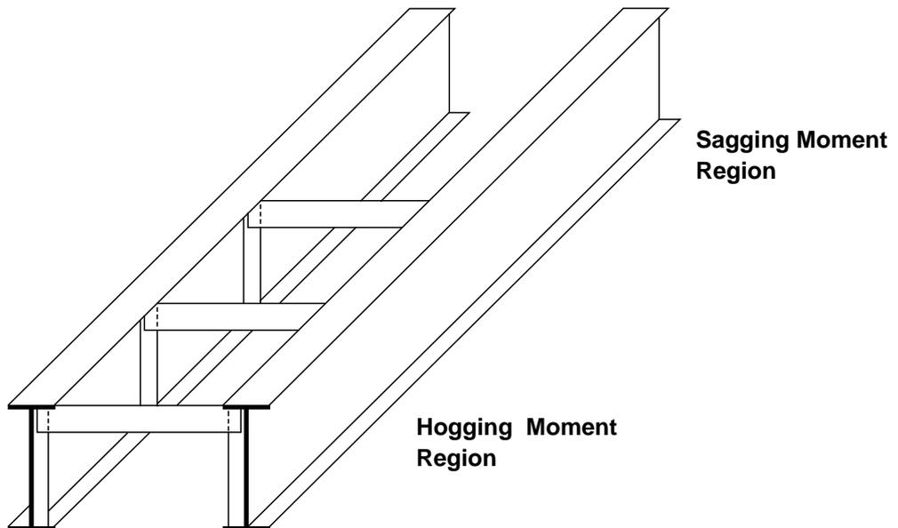
Figure 2 (b) Inverted U-frames at the hogging moment region of a deck type bridge
