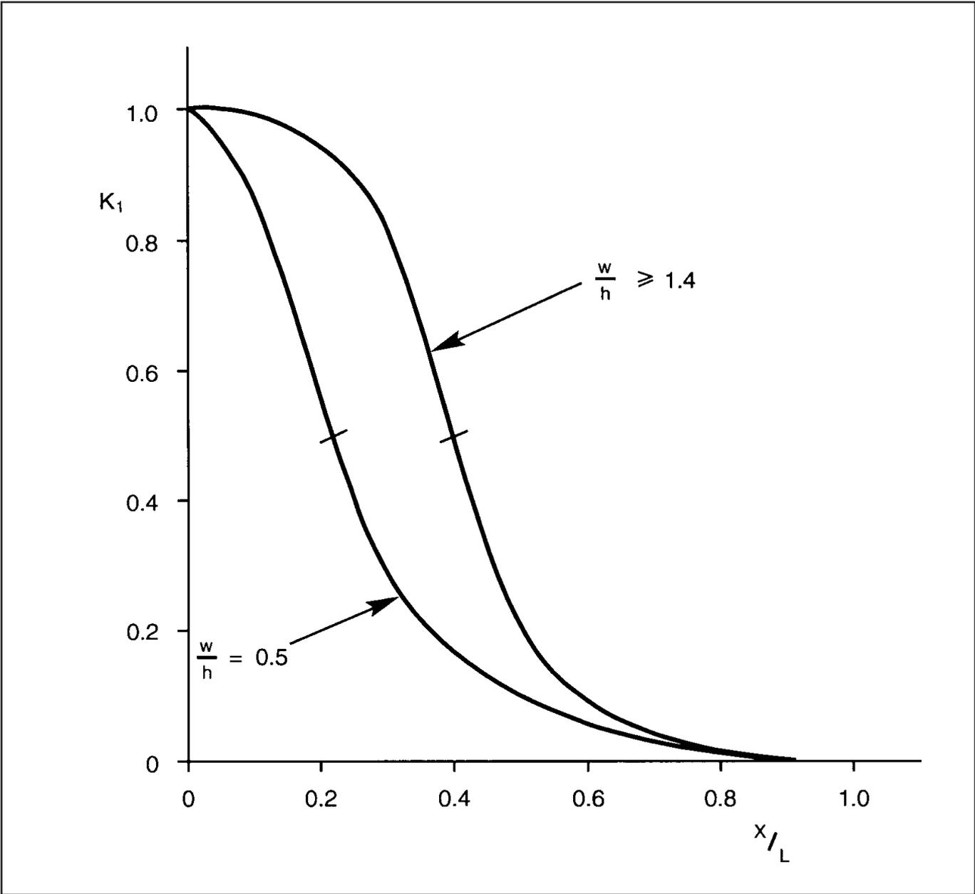
Figure A4 Vertical Subsidence Away From Centre Point or Critical Axis
