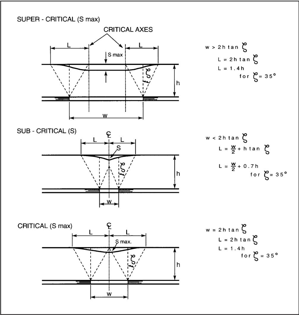
Figure A2 Limit of Curvature of Subsidence Profile (L)
