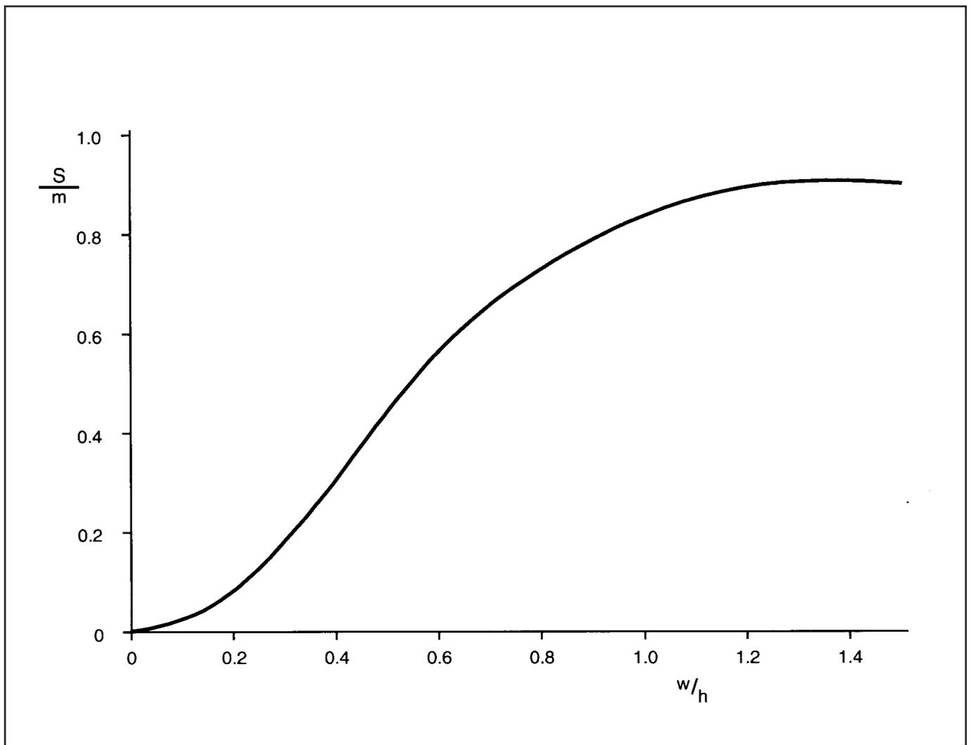
Figure A3 Subsidence at Various Width/Depth Ratios of Extraction
