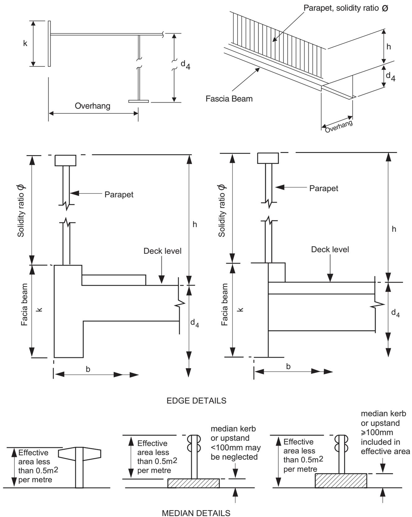
Fig. 2 Bridge deck details for geometric constraints, see 2.3
