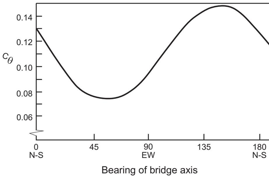
Fig. 4 Factor for orientation of bridge in plan
