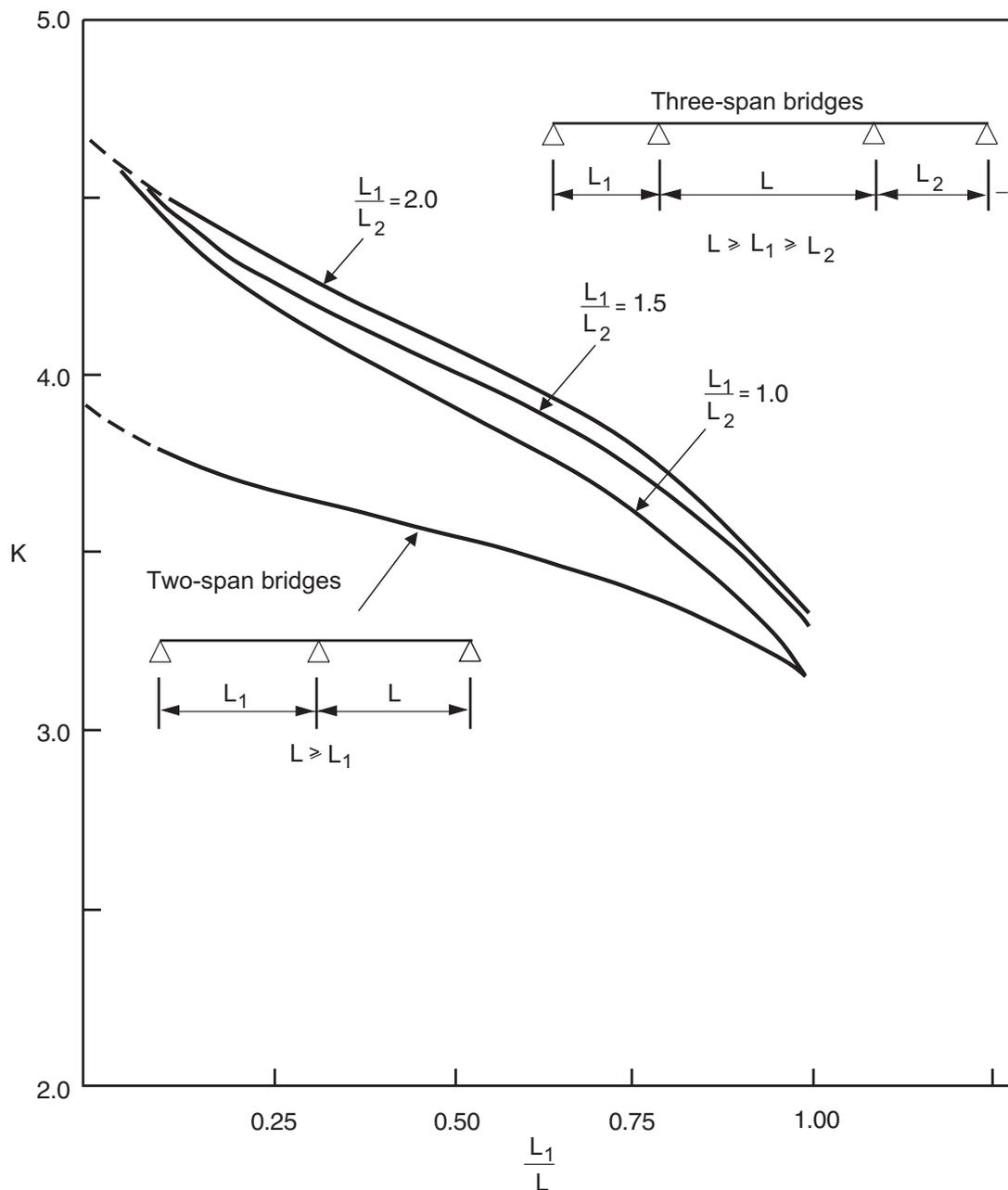
Figure B1 Factor K used for the derivation of fundamental bending frequency
