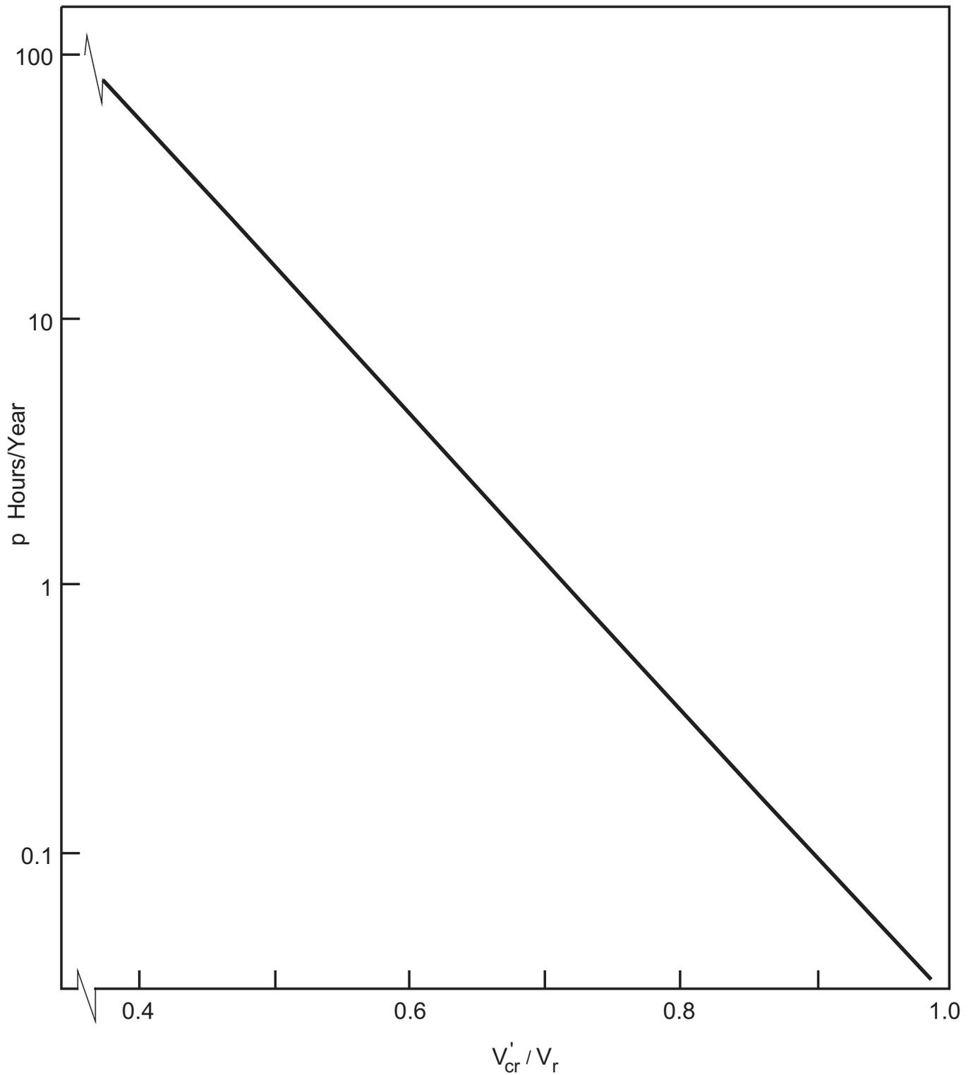
**Fig. 3 Expected frequency of occurrence of critical wind speed
