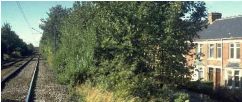
Tyne and Wear Metro Tree Screen Woody vegetation used as a screen needs to be carefully chosen to provide the correct ultimate height and density. Trees alone will ultimately allow open views beneath the crowns
