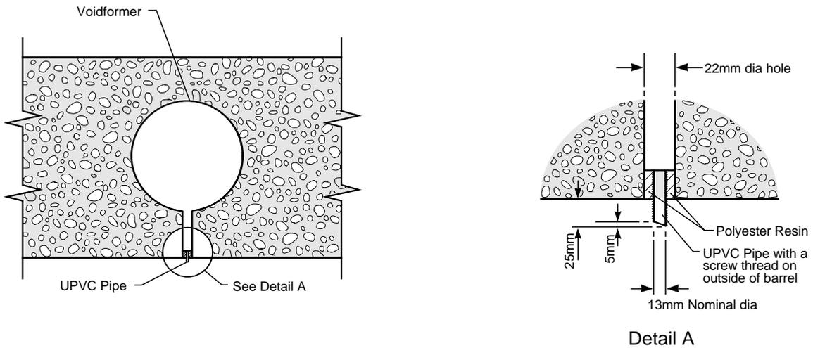
Figure 3: DRAINING OF EXISTING VOIDED SLAB BRIDGES
