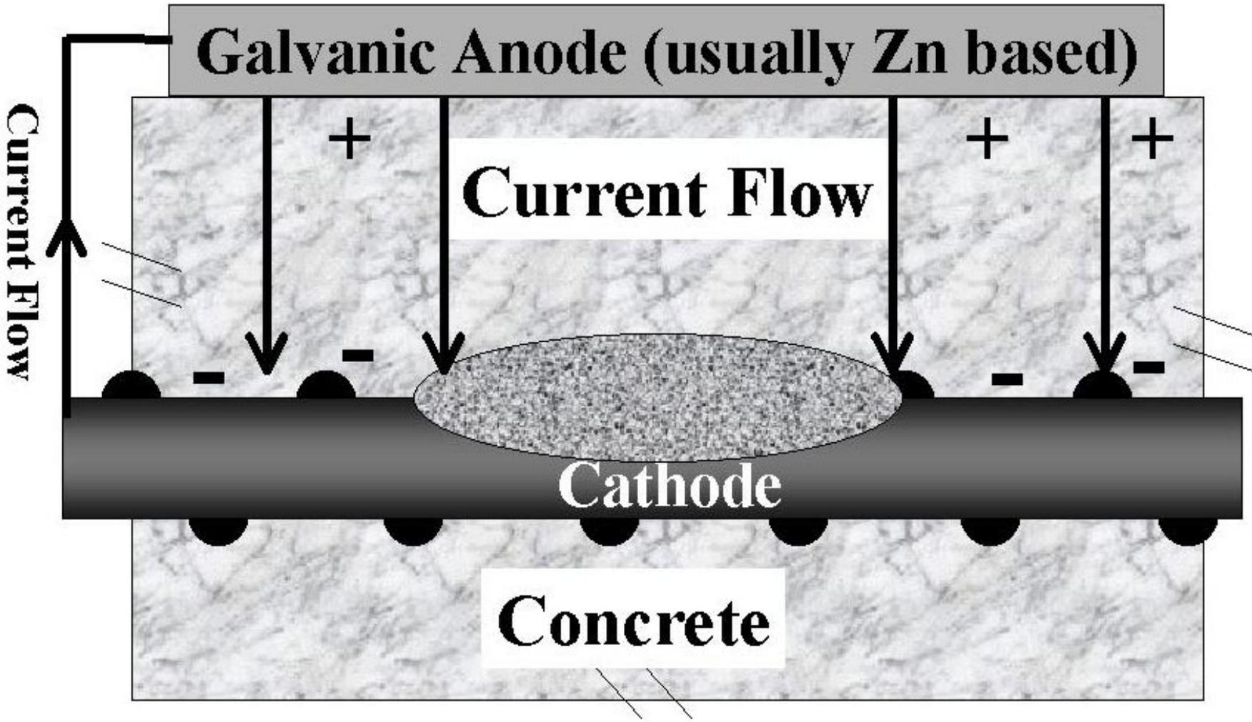
Figure 4. Schematic diagram of galvanic anode cathodic protection system
