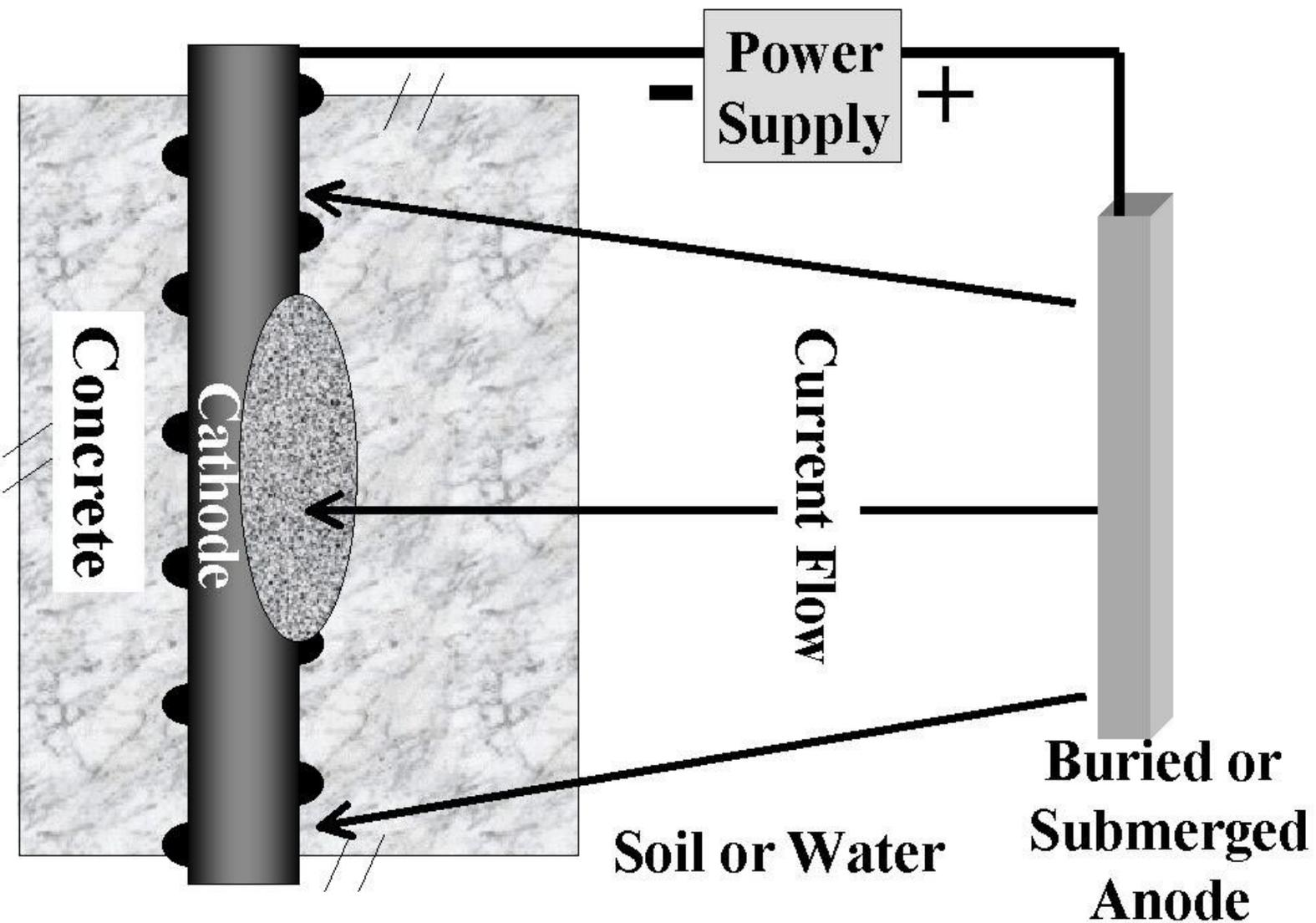
Figure 3. Impressed current cathodic protection schematic for buried or submerged steel in concrete
