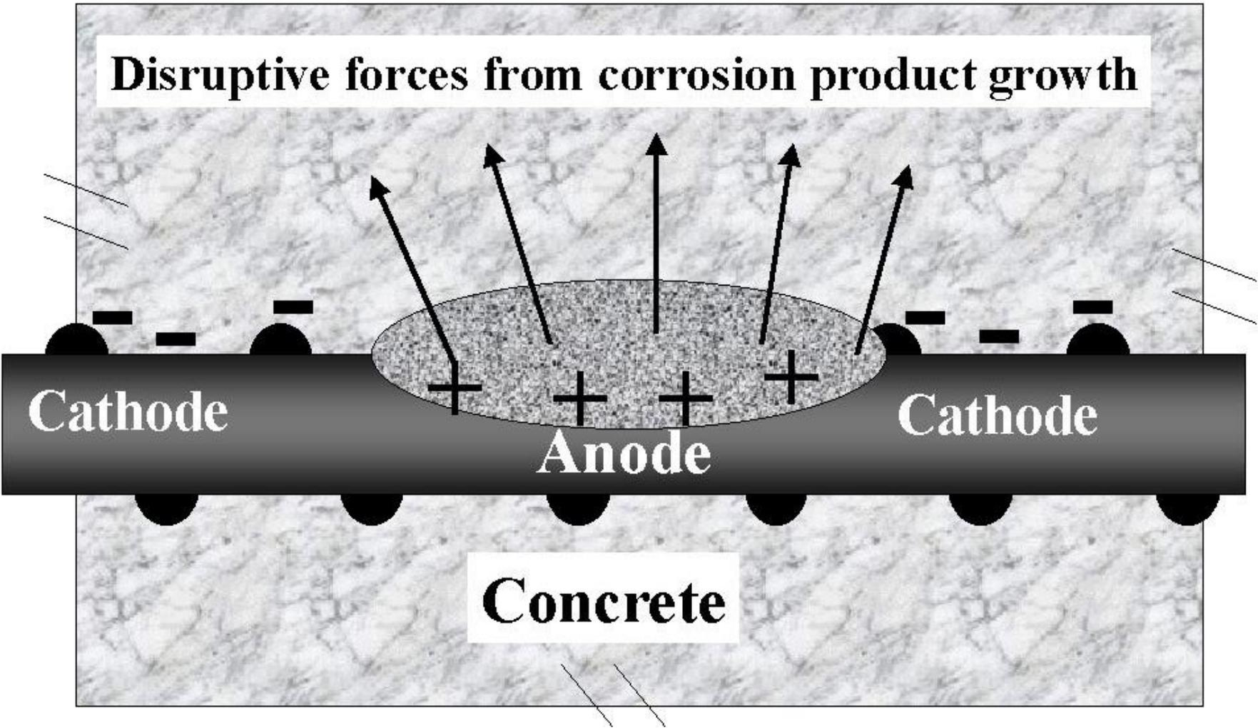
Figure 1. Schematic of embedded reinforcement corrosion cell
