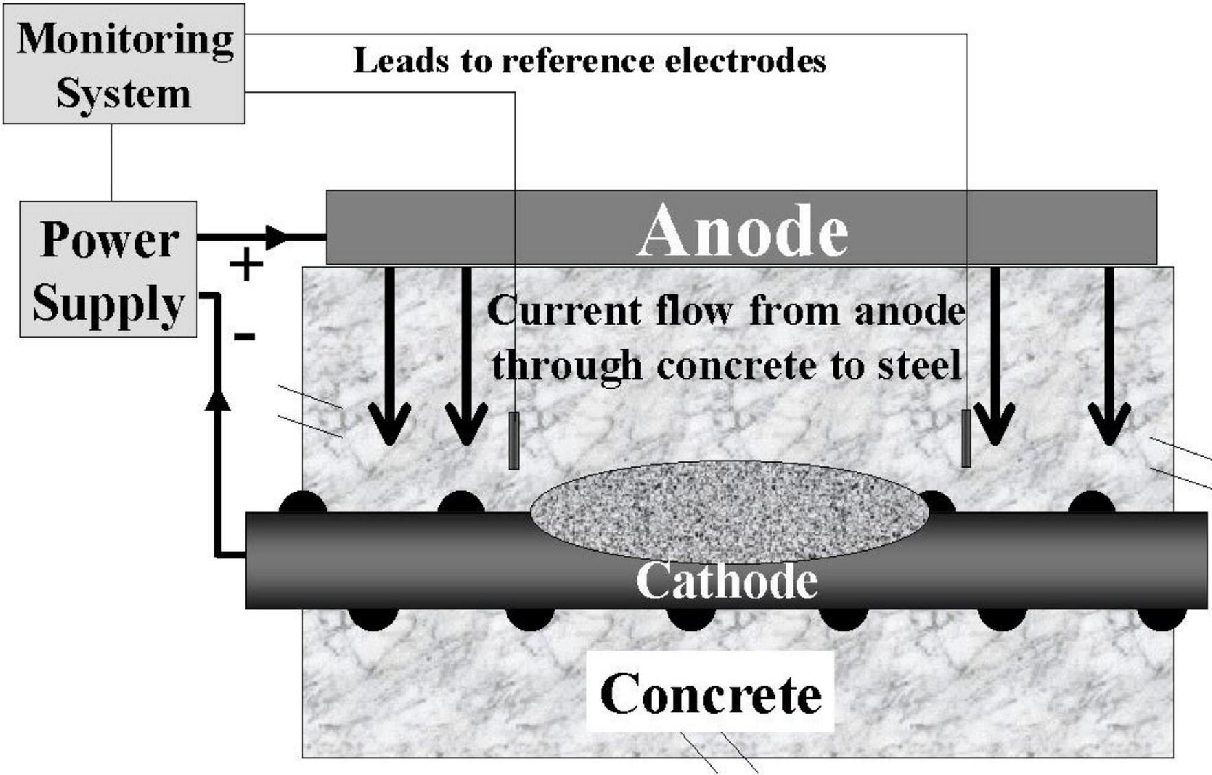
Figure 2. Schematic diagram of impressed current cathodic protection
