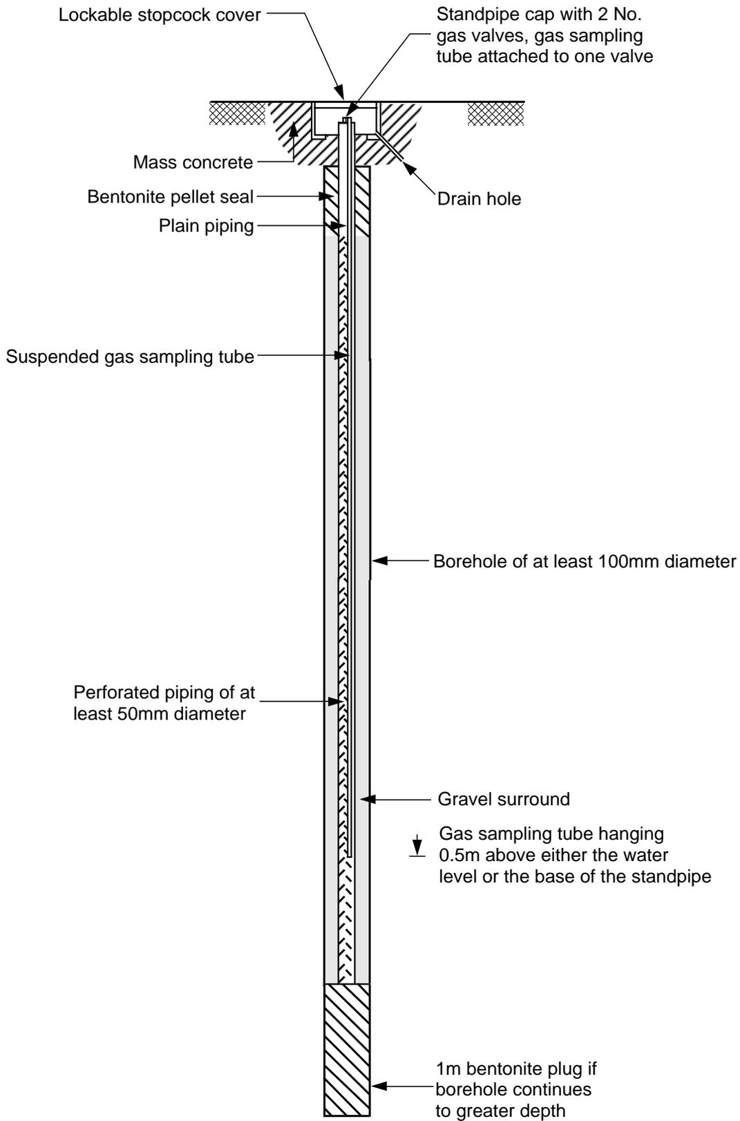
Figure 8/1. Typical details of gas monitoring standpipe
