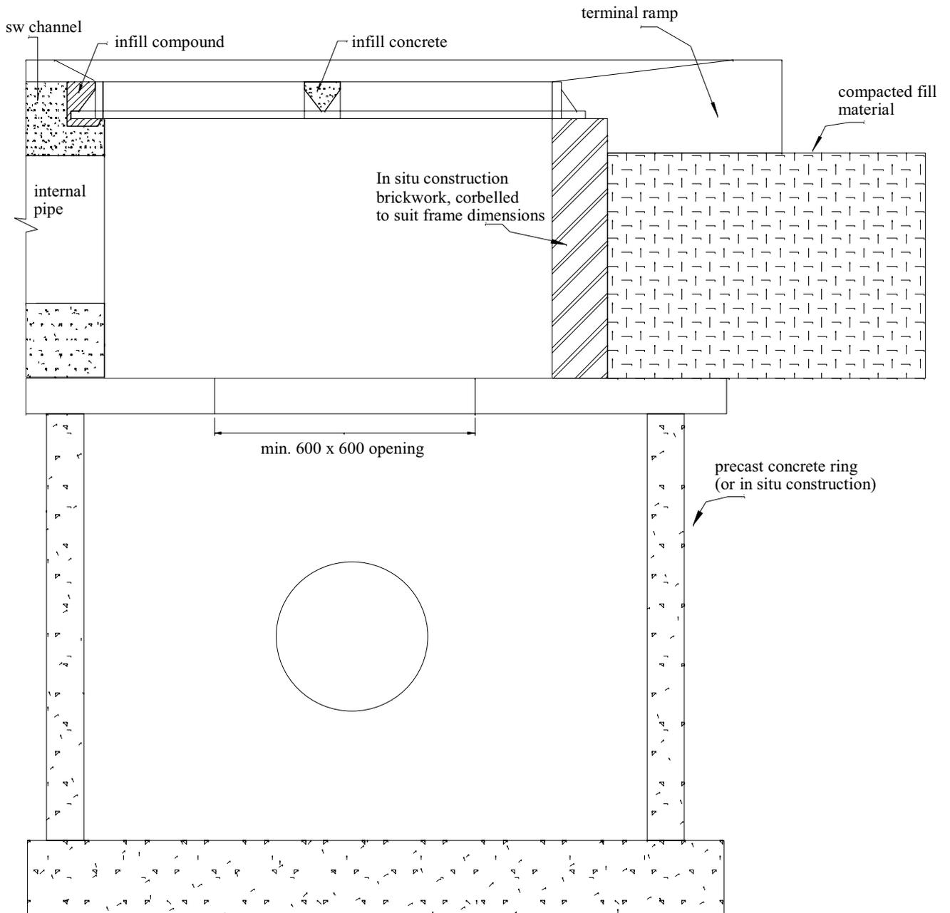
Figure 8b Example of Terminal Outfall - Longitudinal Cross-section
