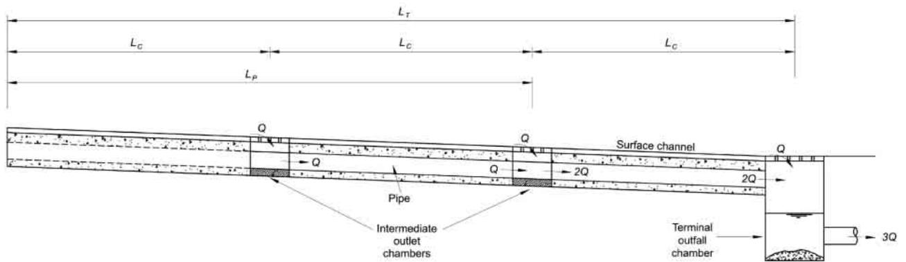
Figure 2 Longitudinal Profile of Combined Surface Channel and Pipe System
