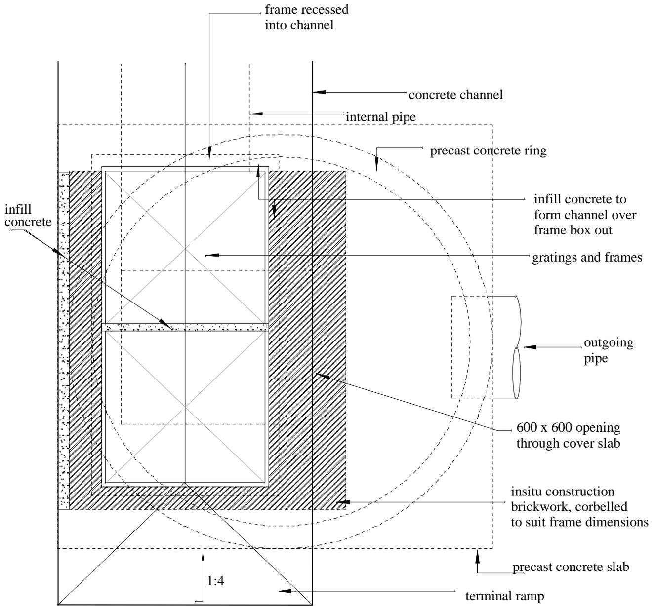
Figure 8a Example of Terminal Outfall - Plan View
