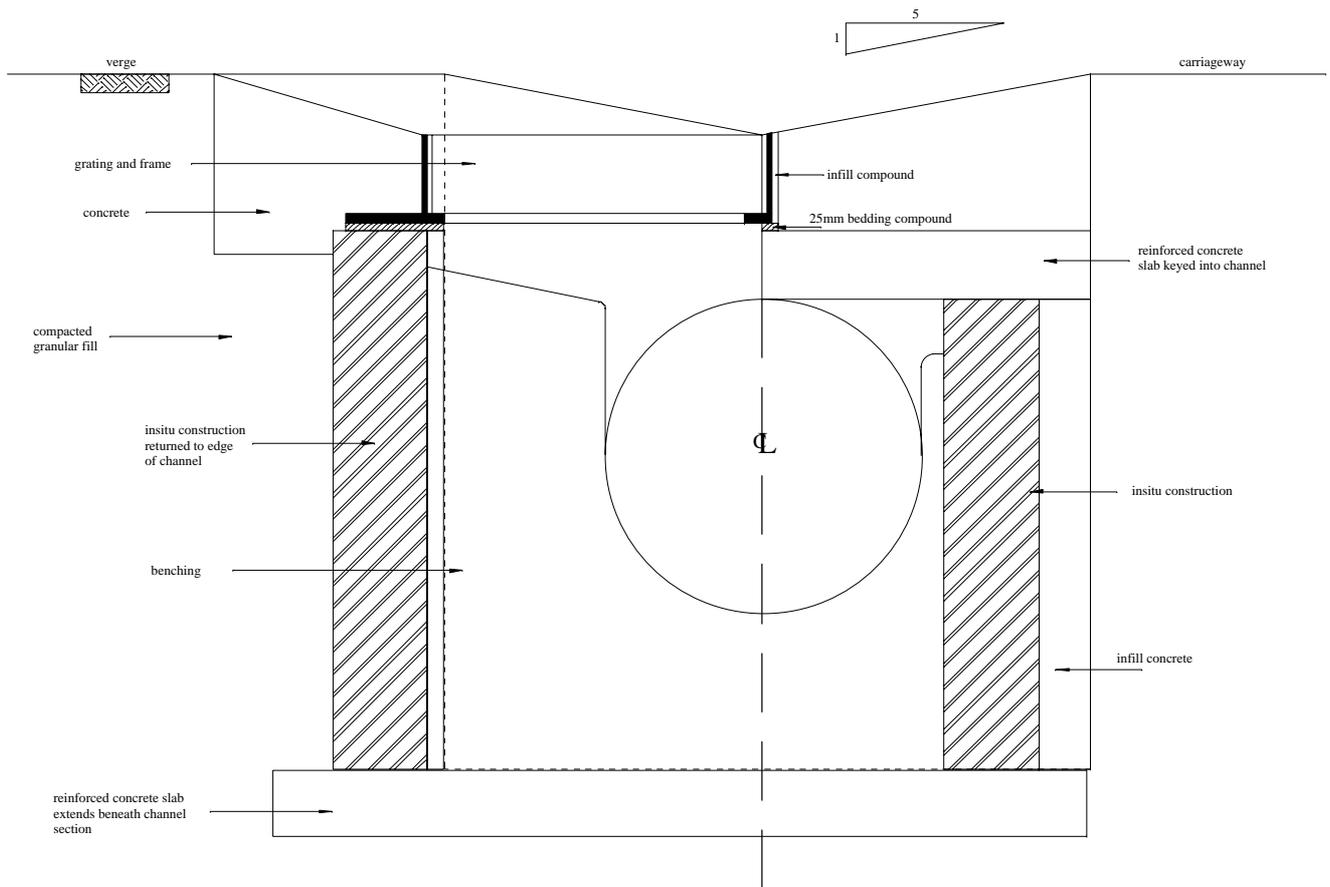
Figure 6 Example of Intermediate Outlet with Off-line Grating
