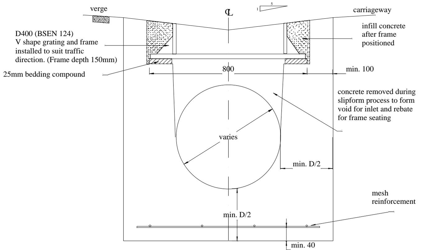
Figure 7 Example of Intermediate Outlet with In-line Grating
