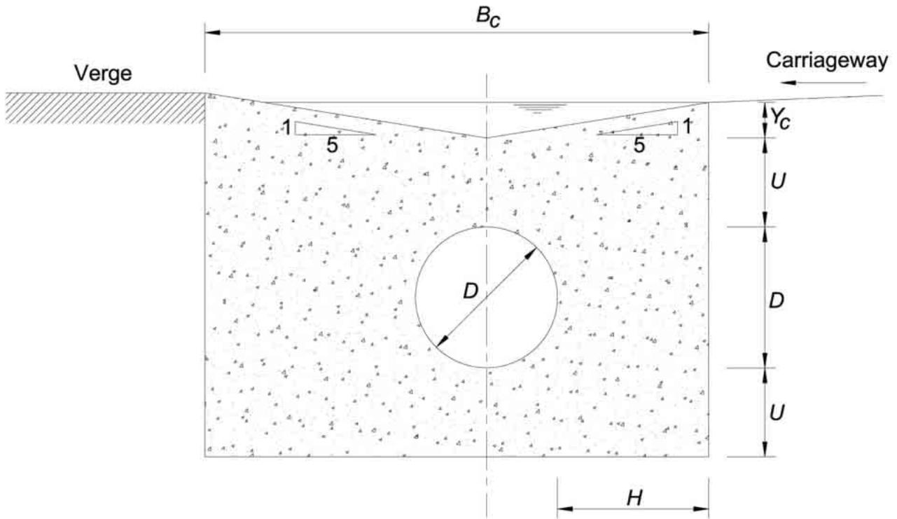
Figure 1 Typical Cross-section of Combined Surface Channel and Pipe System
