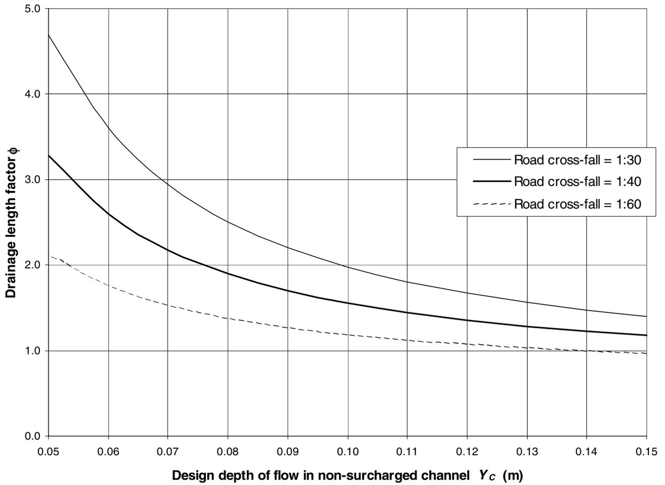
Figure 5 Drainage Length Factor  $\phi$  for Triangular Channels with Surcharged Width of  $B_s = 1.5\text{m}$
