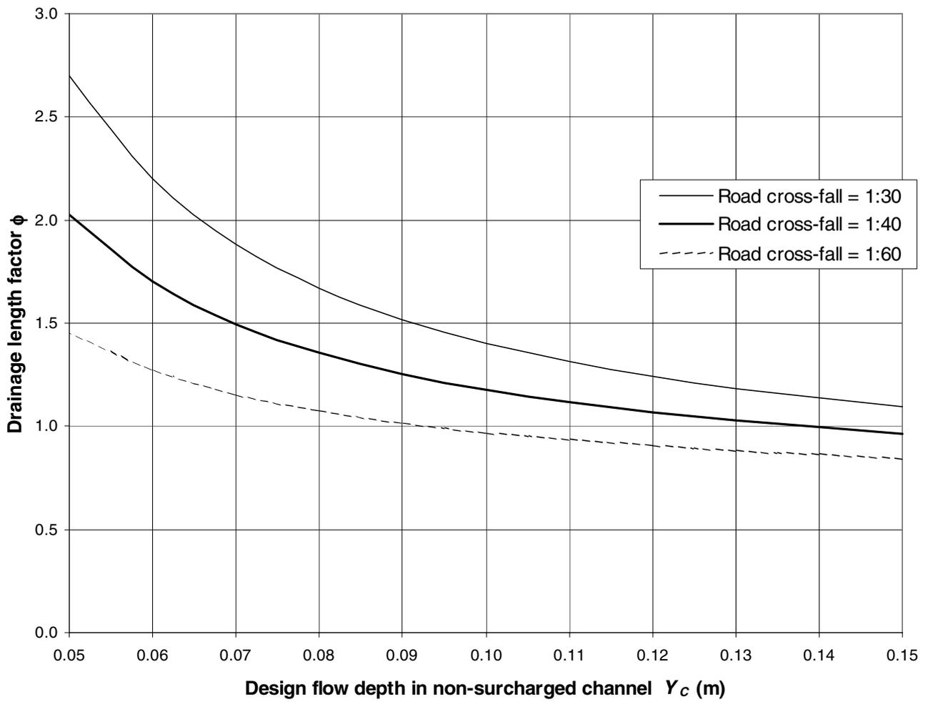
Figure 4 Drainage Length Factor  $\phi$  for Triangular Channels with Surcharged Width of  $B_s = 1.0\text{m}$
