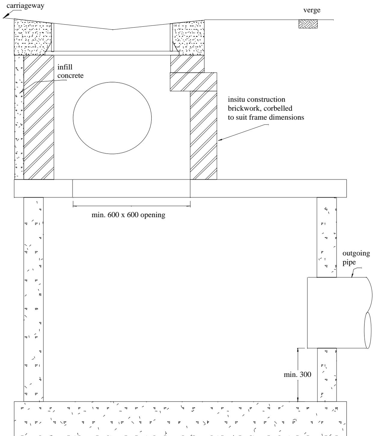
Figure 8c Example of Terminal Outfall - Transverse Cross-section
