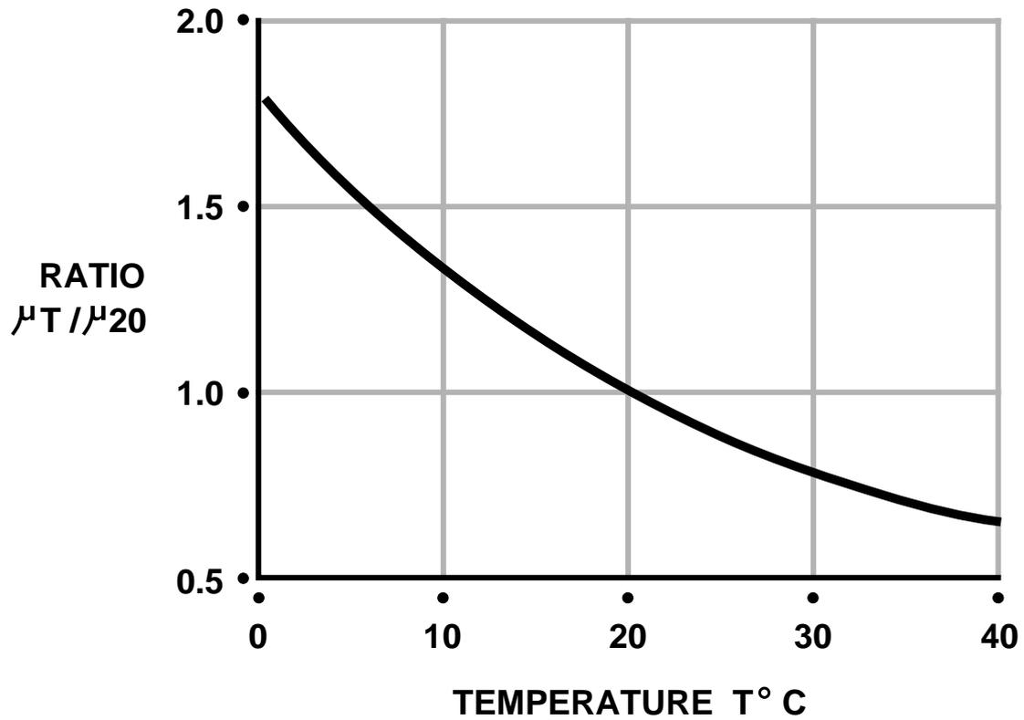
Fig.2 Relationship between dynamic viscosity of water and temperature (based on data from Kaye and Laby. 1986)
