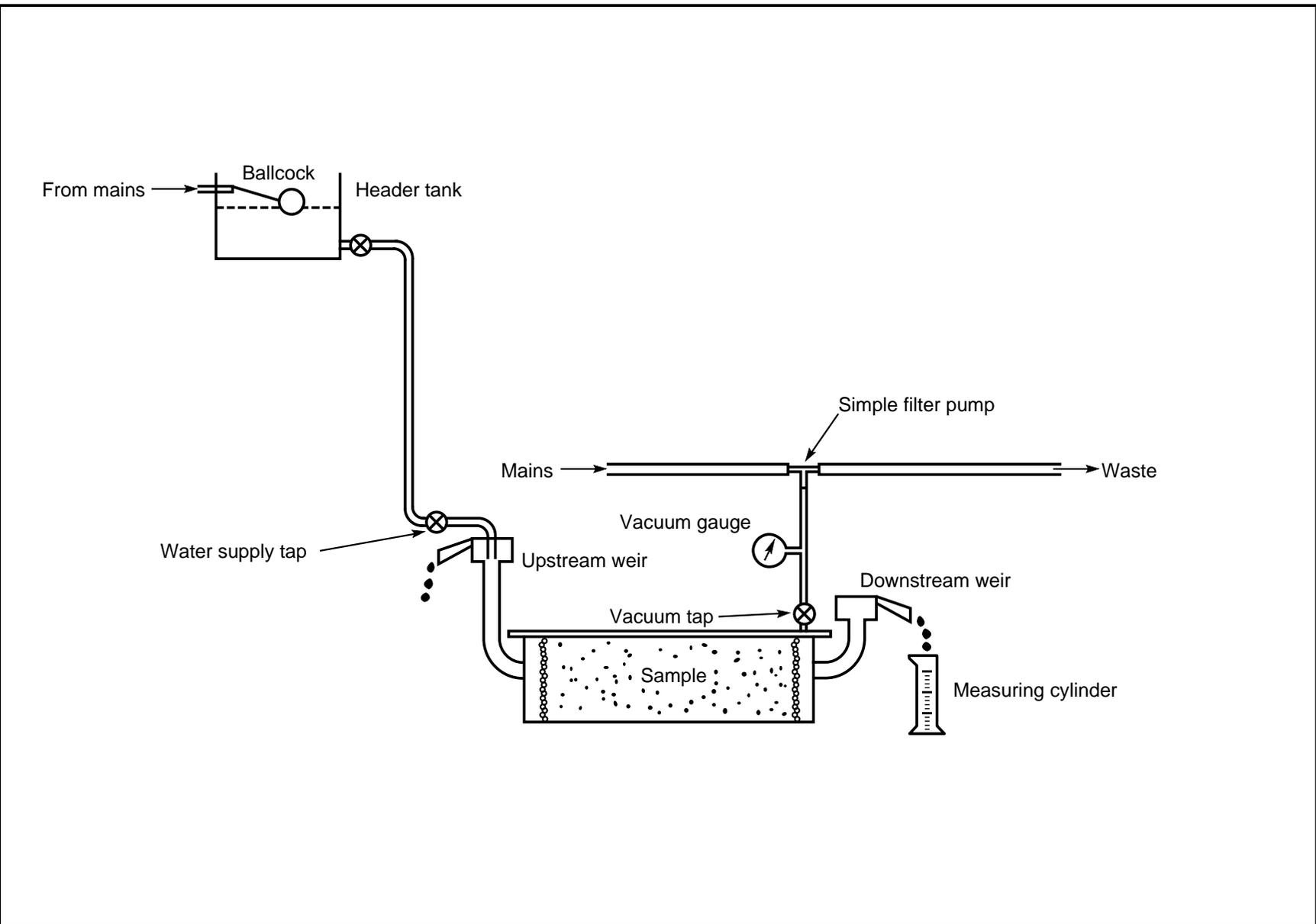
Fig 1 Schematic diagram of apparatus
