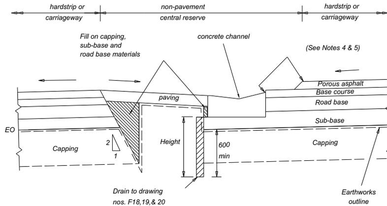
**TYPE Sk3A - STANDARD CONCRETE CHANNEL
