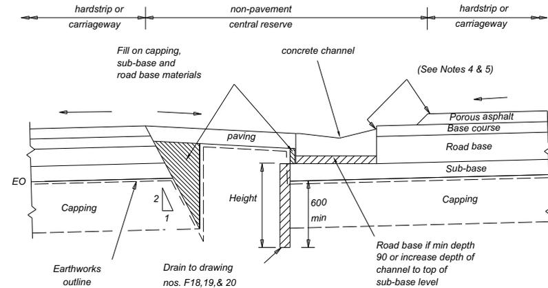
**TYPE Sk3C - STANDARD CONCRETE CHANNEL
