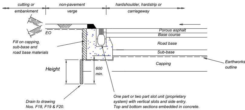
**TYPE Sk5A - LINEAR DRAINAGE CHANNEL WITH TOP GRATING AND ADDITIONAL SIDE ENTRY OPENINGS**
