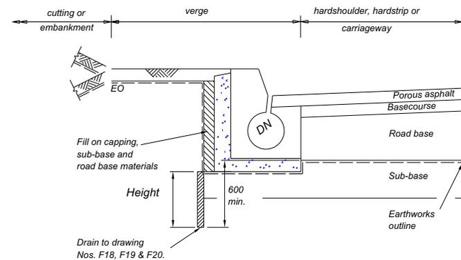
**TYPE Sk5D - COMBINED LINEAR SLOT DRAINAGE CHANNEL AND KERB SYSTEM**
