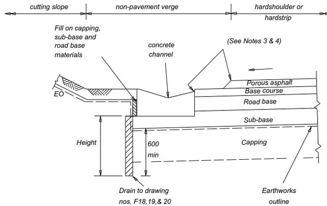
**TYPE Sk4A - STANDARD CONCRETE CHANNEL IN VERGE
