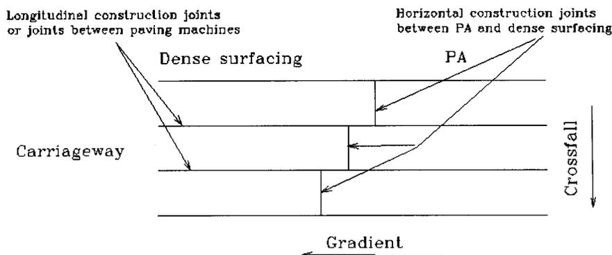
**Figure 3.2 Plan showing Staggered Lane Ends for PA**
