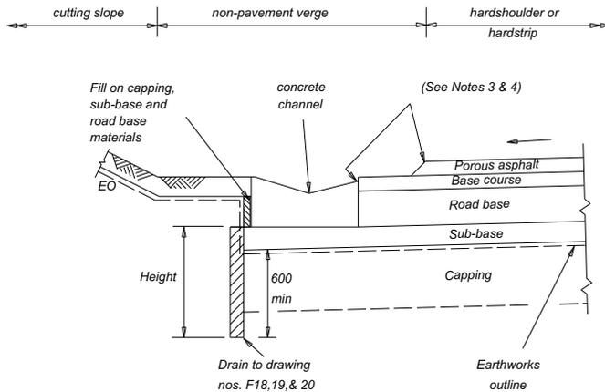
**TYPE Sk4B - STANDARD CONCRETE CHANNEL IN VERGE
