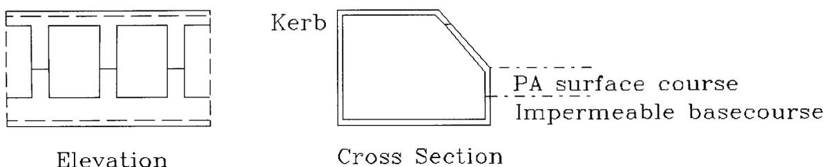
Figure 5.1 Proposed Combined Drainage and Kerb System
