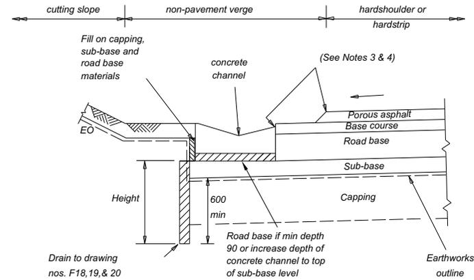
**TYPE Sk4C - STANDARD CONCRETE CHANNEL IN VERGE
