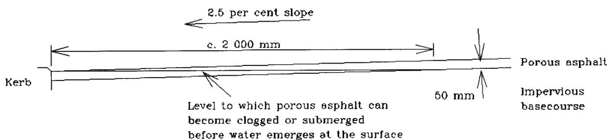
Figure 3.1 Clogging Effect on an Impermeable Kerb
