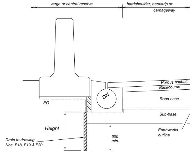
**TYPE Sk5C - LINEAR SLOT DRAINAGE CHANNEL FOR USE IN CONJUNCTION WITH VERTICAL CONCRETE BARRIER**
