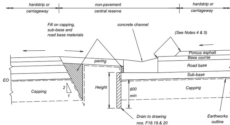
**TYPE Sk3B - STANDARD CONCRETE CHANNEL
