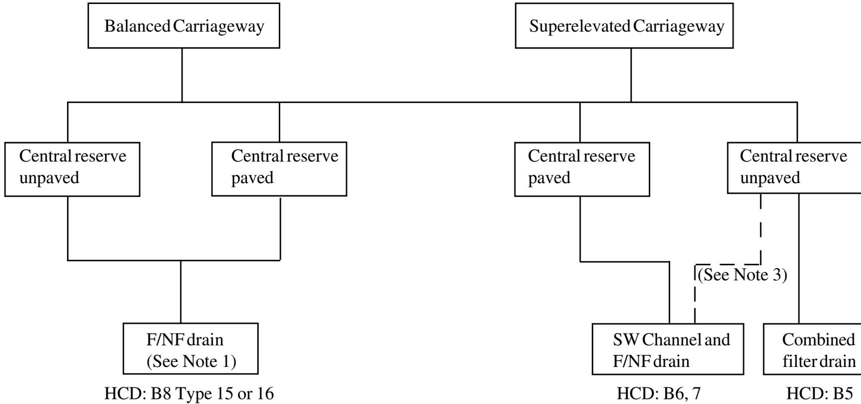
Figure 3.2: Recommended Design Selection Central Reserve Drainage
