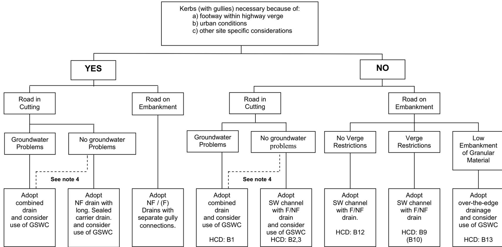
Figure 3.1: Recommended Design Selection Verge-Side Edge Drainage
