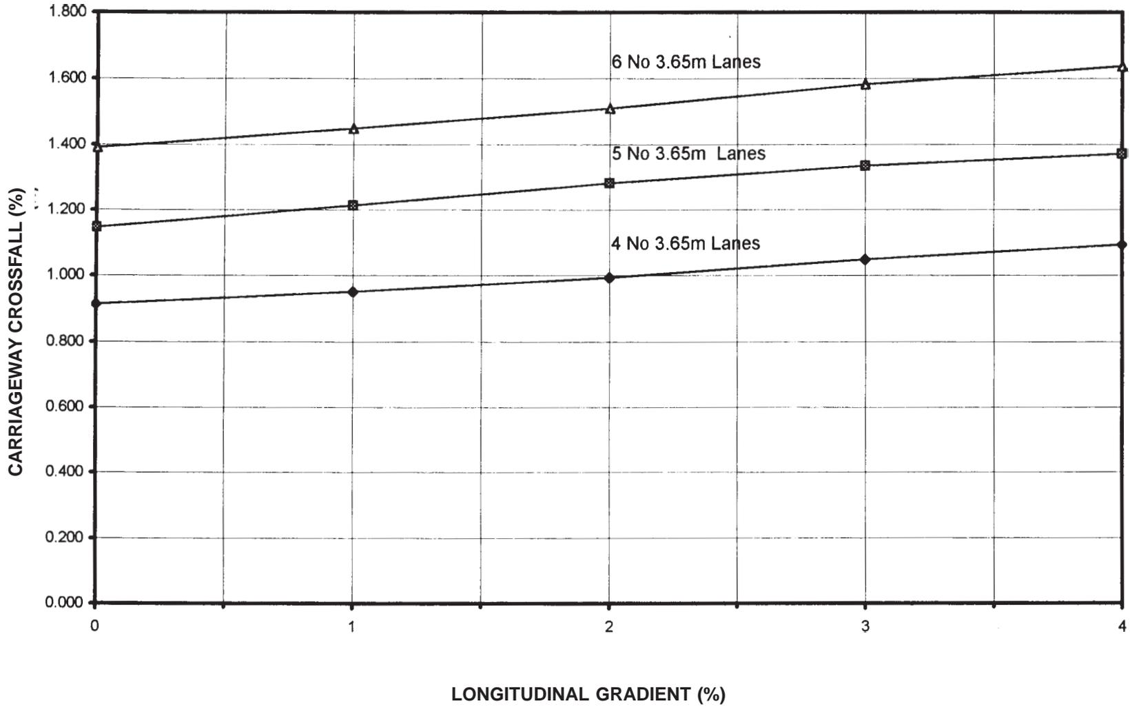
Note: The combinations of Longitudinal Gradient and Crossfall below the curves are likely to allow greater depths of water than are normally acceptable on road layouts and should be avoided.
