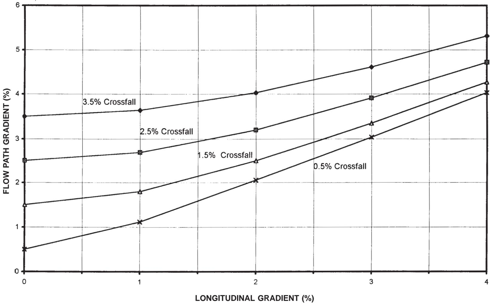
FIG 2.3 EFFECT OF GEOMETRIC DESIGN ON DRAINAGE
