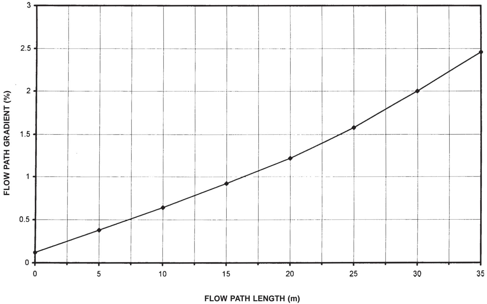
Note: The combinations of Flow Path Length and Flow Path Gradient below the curve are likely to allow greater depths of water than are normally acceptable on road layouts and should be avoided.
