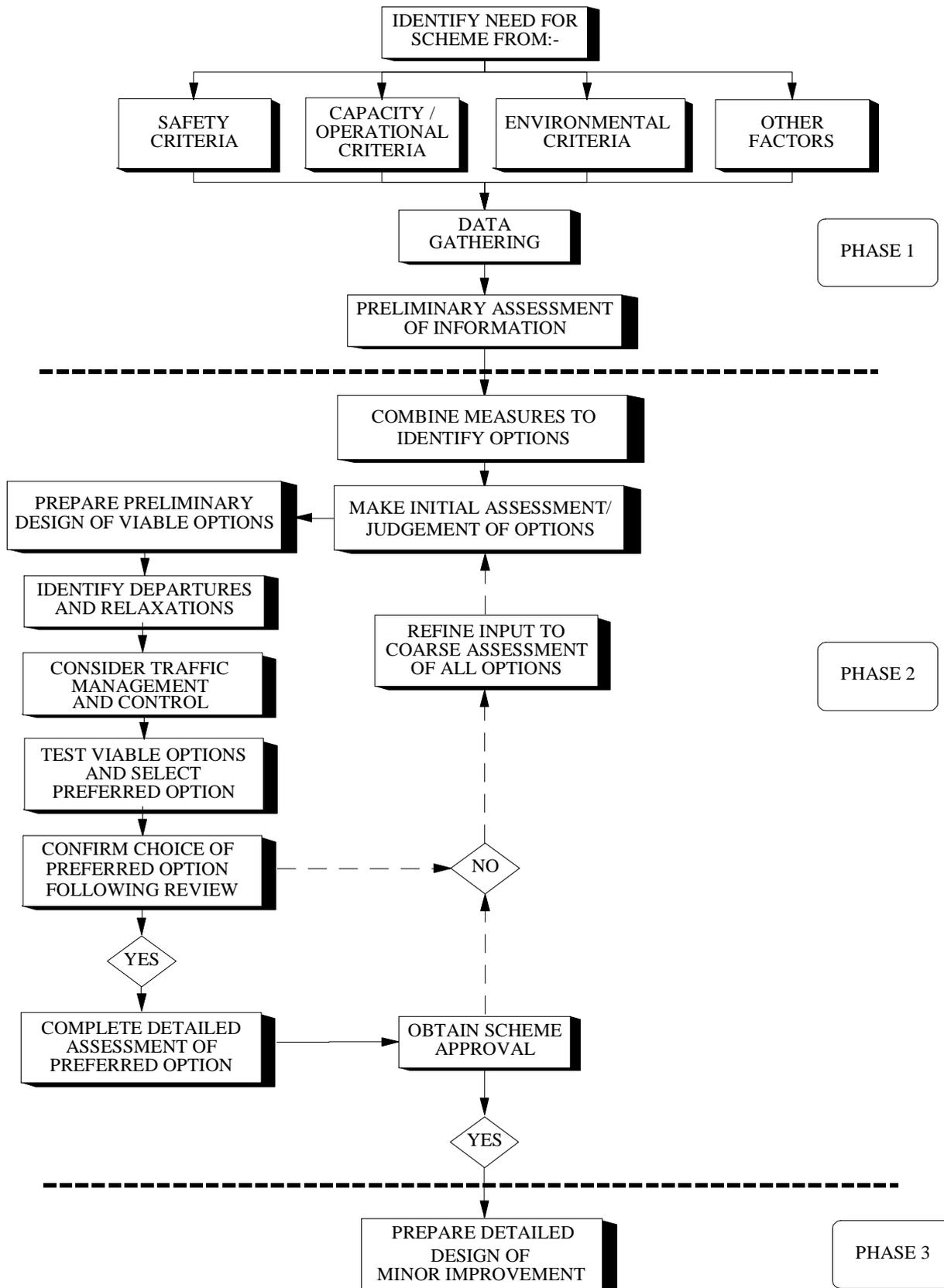
Figure 3/1: Design Procedure
