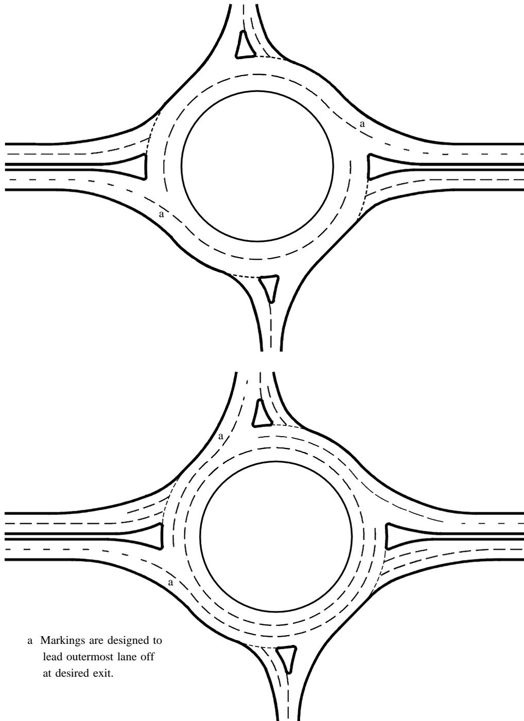
a Markings are designed to lead outermost lane off at desired exit.
