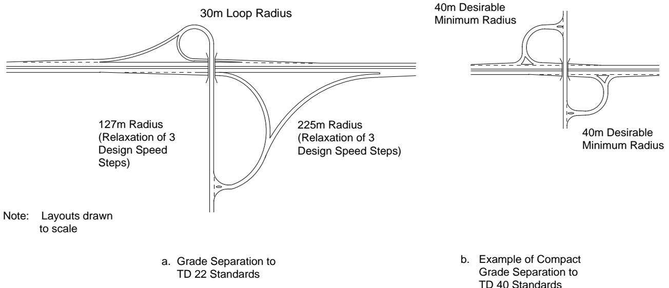
Figure 1/1 Examples of the range of Grade Separations
