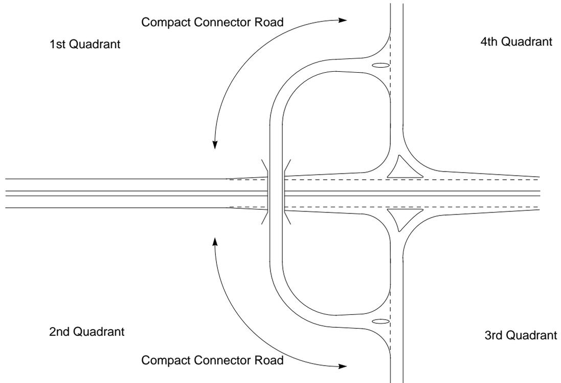
Figure 7/3 Compact Grade Separation for 4 Arm Junction, Showing Merge and Diverge Tapers
