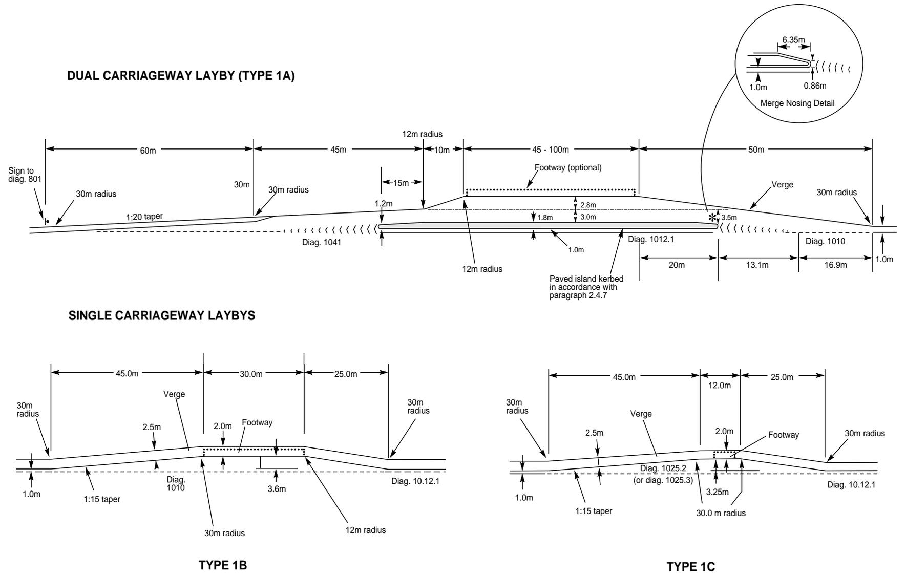
Fig 1 - GEOMETRIC LAYOUT OF 'LAYBYS'
