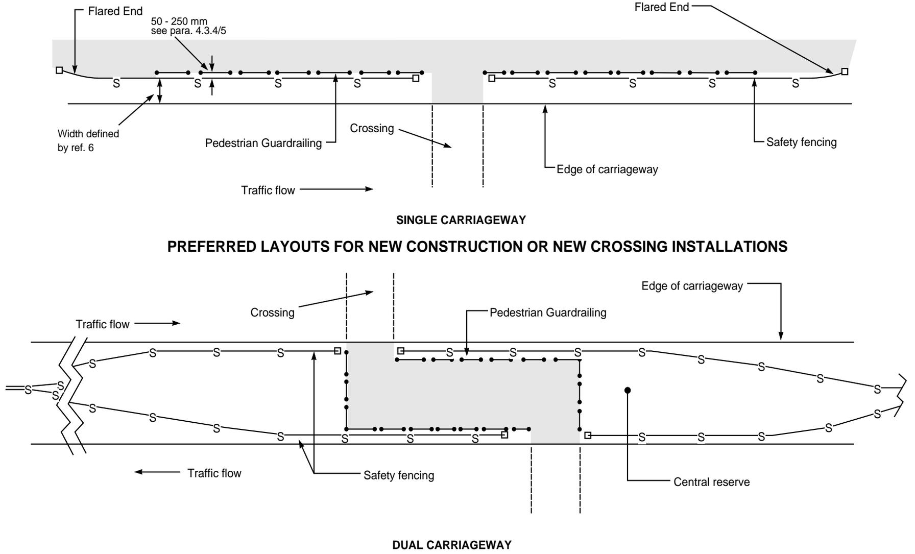
**FIG.5 PEDESTRIAN GUARDRAILING - PROTECTION BY SAFETY FENCING**
