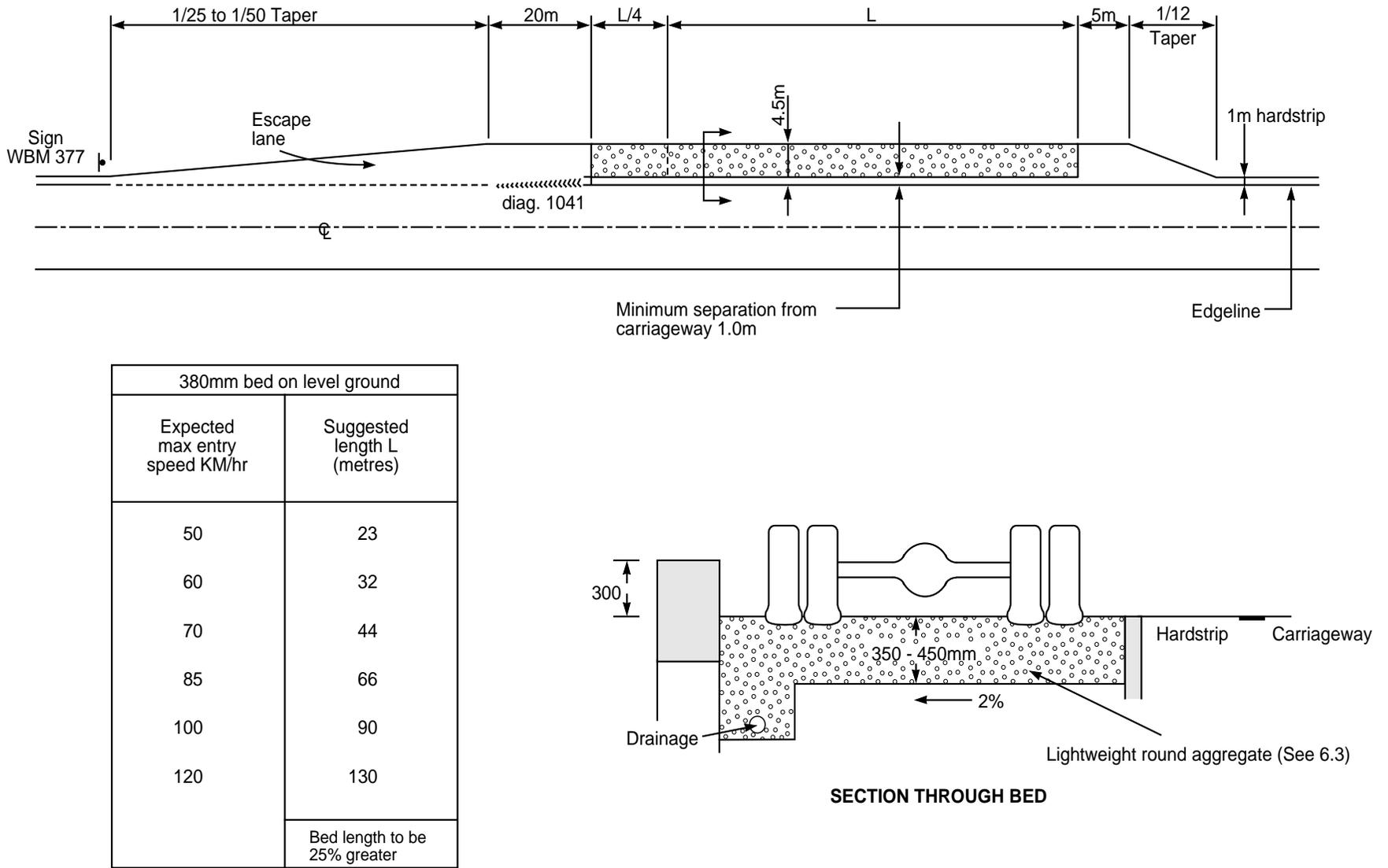
**FIG.7 LAYOUT OF ARRESTER BED ADJACENT TO CARRIAGEWAY**
