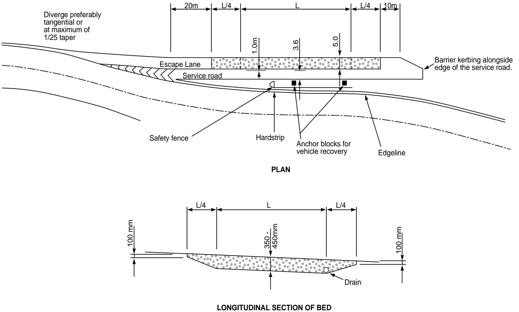
**FIG.8 SUGGESTED LAYOUT OF ARRESTER BED REMOTE FROM CARRIAGEWAY**
