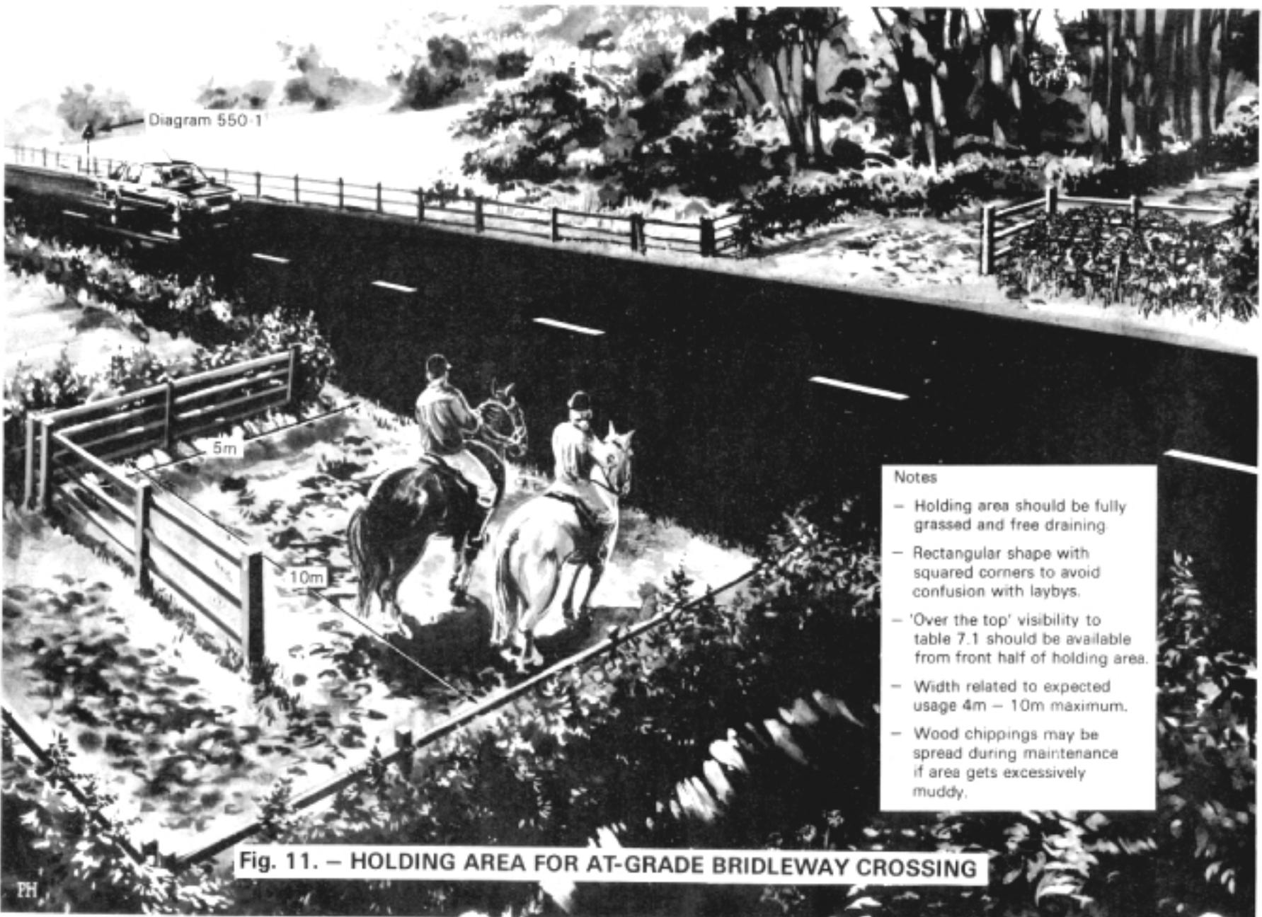
Fig. 11. - HOLDING AREA FOR AT-GRADE BRIDLEWAY CROSSING
