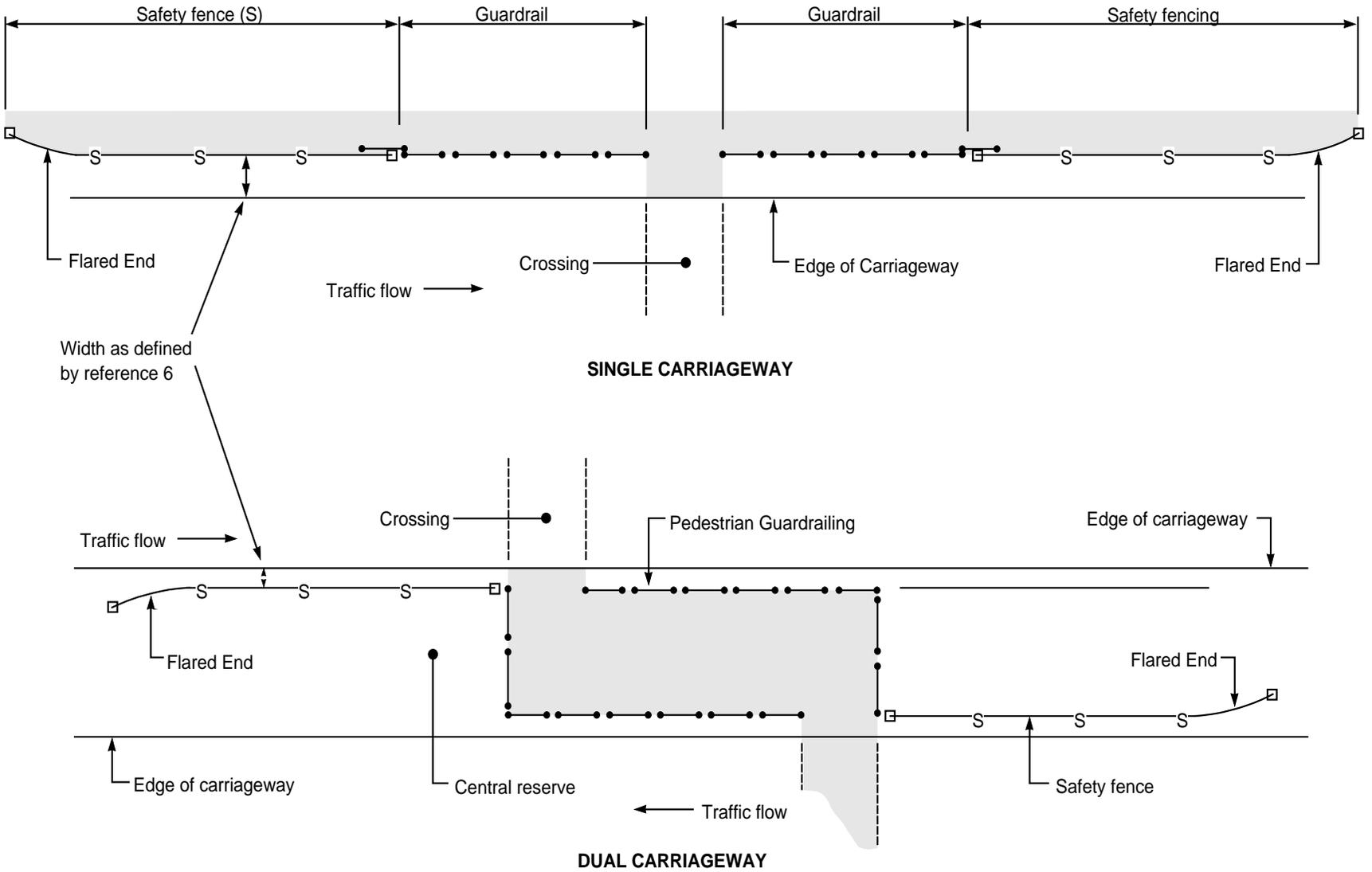
**Figure 6 Pedestrian Guardrailing - Protection by Safety Fencing**
