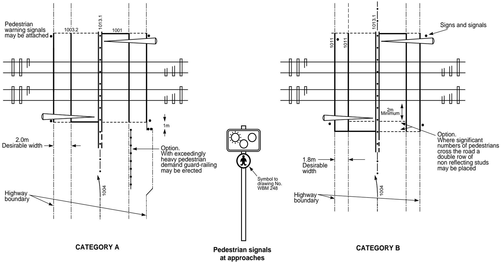
FIG.12 LAYOUT OF RAILWAY LEVEL CROSSINGS - SHEET 1
