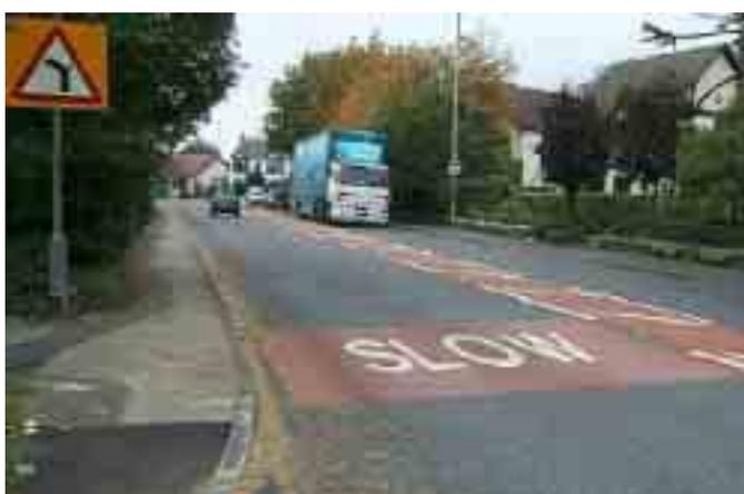
3.16 Coloured surface patches are commonly used as part of gateways or to emphasise the presence of particular traffic calming features. They are generally laid across the full width of the carriageway and are typically 8-12m long. The choice of colour is important. Red surfacing will have high initial visual impact but
