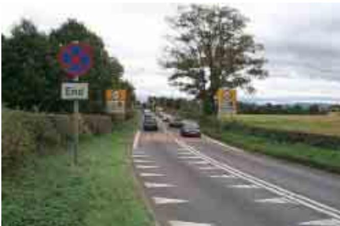
3.7 Gateways are a common feature of most trunk road traffic calming schemes. They are designed to highlight to drivers that they are entering an area of changed road use e.g. a village. They may involve some form of physical measures, carriageway markings, signing, often incorporating the name of the village, and a change of speed limit.
