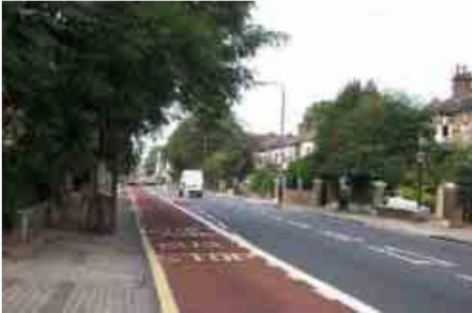
3.28 Allocating carriageway for the specific use of a particular type of vehicle such as a bus or cycles can act as a calming measure by reducing the space available for other motorised users. This technique is most likely to be used in, or on the approaches to, larger settlements. Cycle lanes should not be put in solely as a traffic calming measure where there is no demand or suppressed demand. Drivers can become accustomed to empty lanes and start ignoring them.
