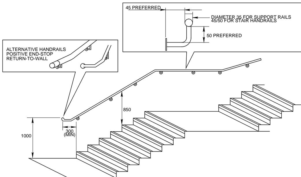
Figure 4 Handrailing details
