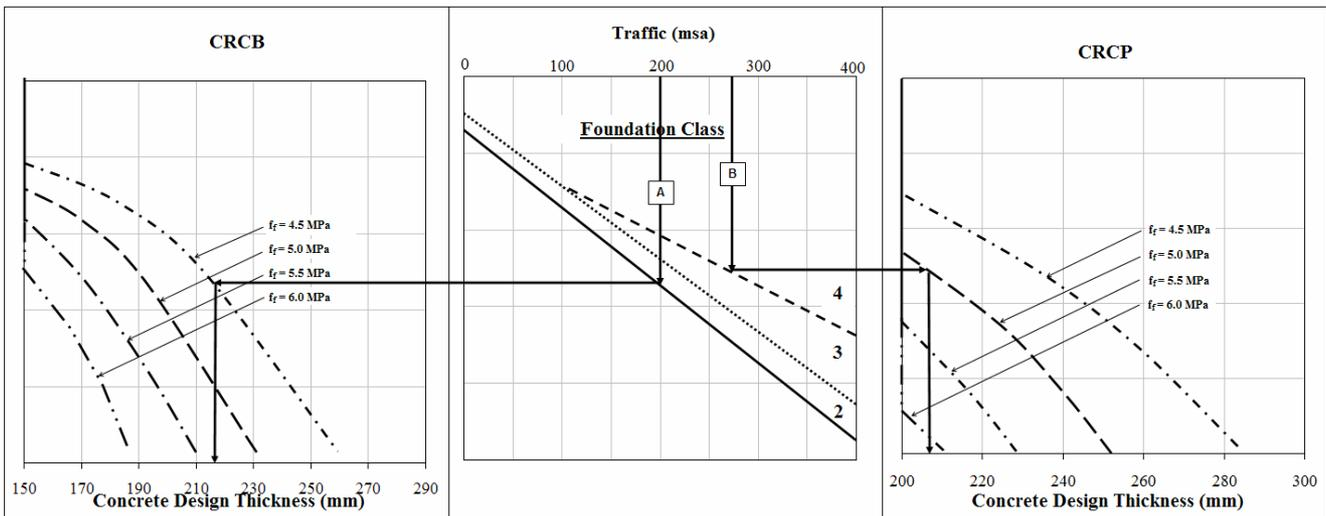
Designs for jointed concrete pavements are based on work contained in TRL Report RR 87 (1987) and are related to the compressive strength of the concrete.
