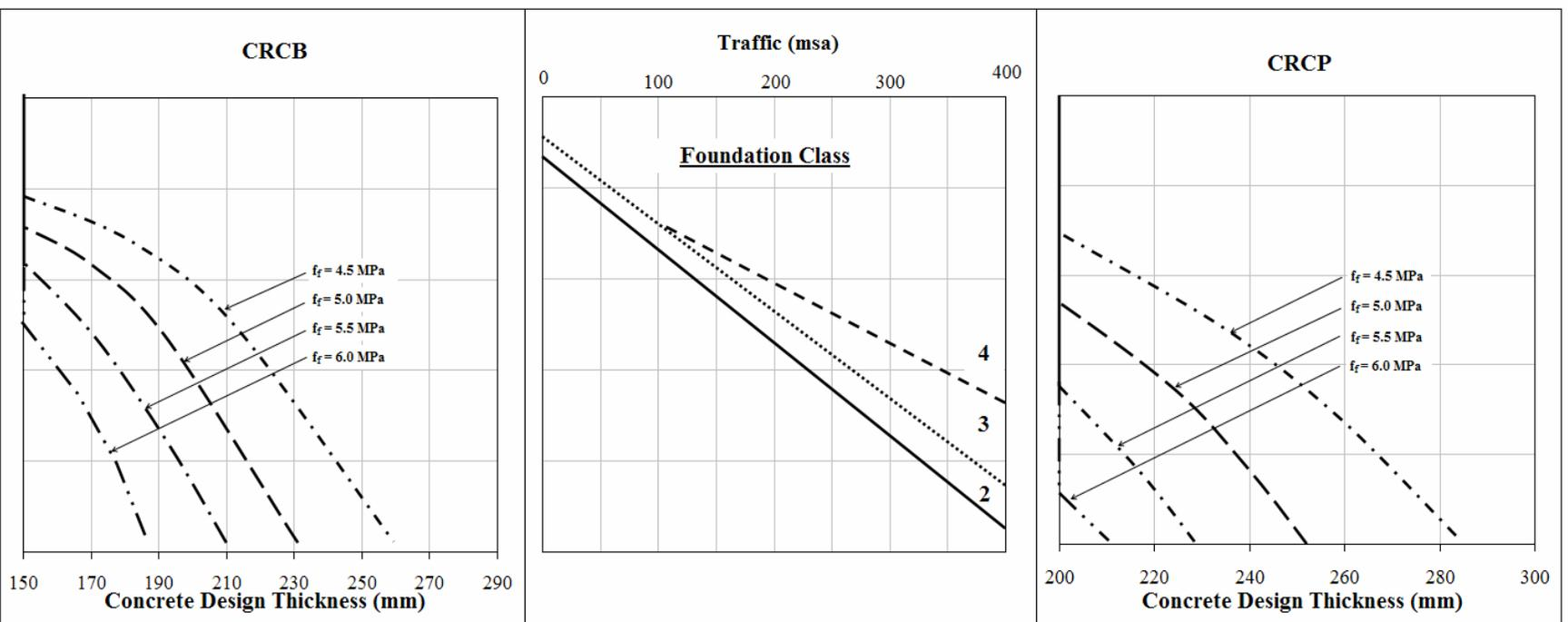
Figure 2.2: Design Thickness for Rigid (Continuous) Pavements
