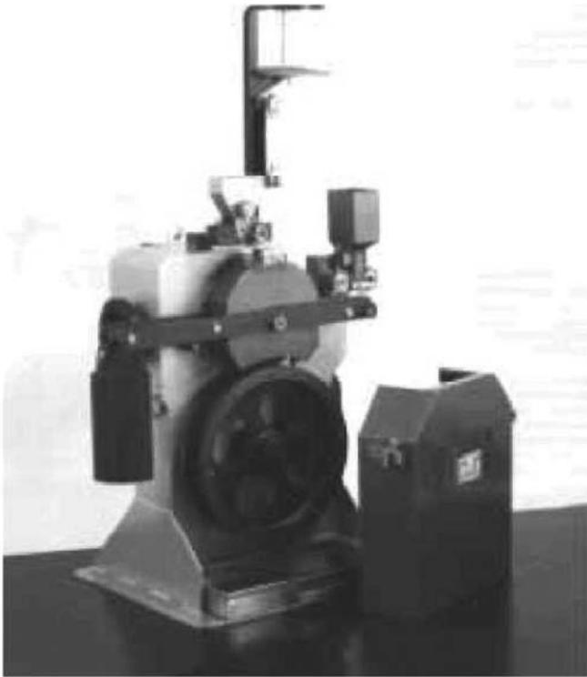
Figure 3.2: Accelerated Polishing Machine
