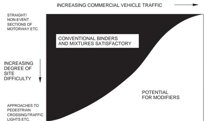
**Figure 3.1 : The Need for Modifiers in Mixtures at Difficult Sites and at High Traffic Intensity.**
