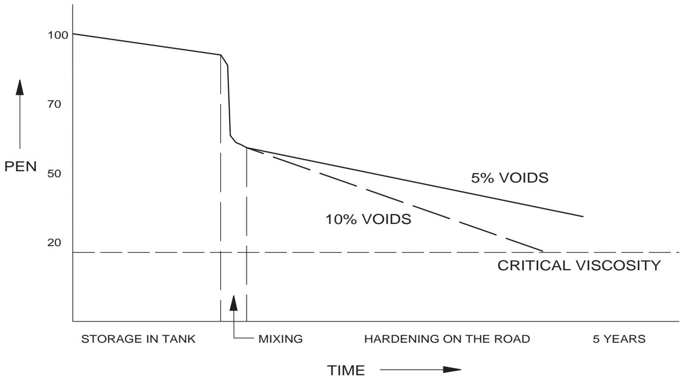
**Fig 3.6 : Changes in Penetration of Conventional 100 pen Bitumen with Time, for Mixtures of differing Voids Contents**
