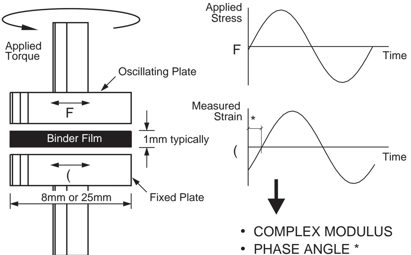
3.2 : Essential Parts of Dynamic Shear Rheometer and Definition of Phase Angle  $\delta$
