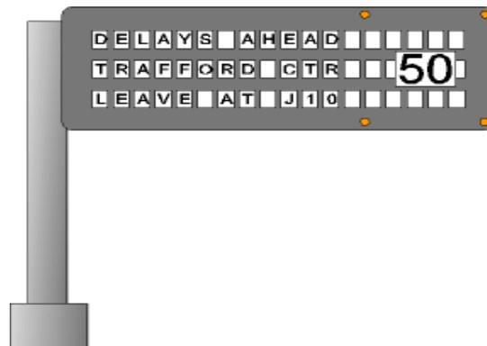
Figure 2 - Motorway Signal Mark 3 (MS3)
