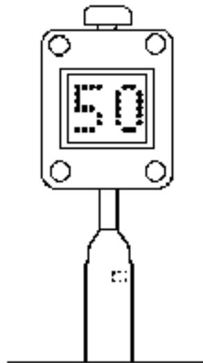
Figure 1 - Post Mounted Matrix Signal (MS1)
