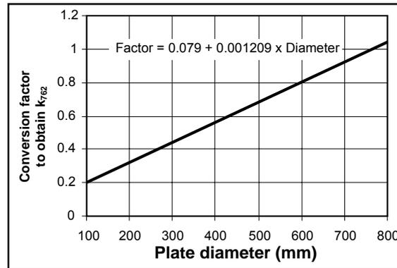
**FIGURE 7.4 Conversion Factors for Smaller Plate Sizes**
