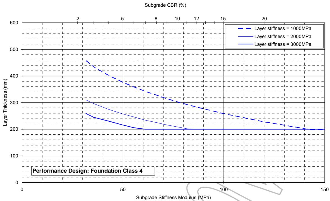
**FIGURE 4.5 Class 4 Designs – Single Foundation Layer**
