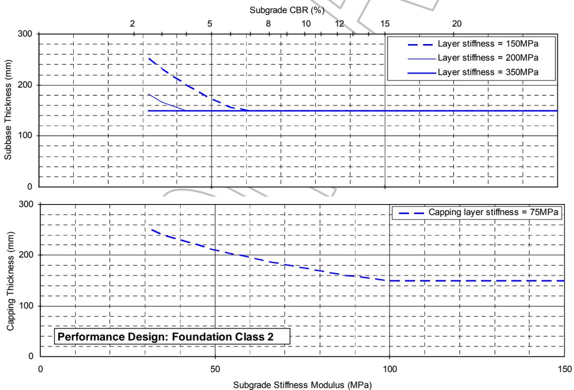
**FIGURE 4.6 Class 2 Designs – Subbase on Capping**
