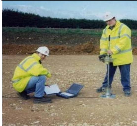
**FIGURE 7.5 Lightweight Dynamic Plate Test**
