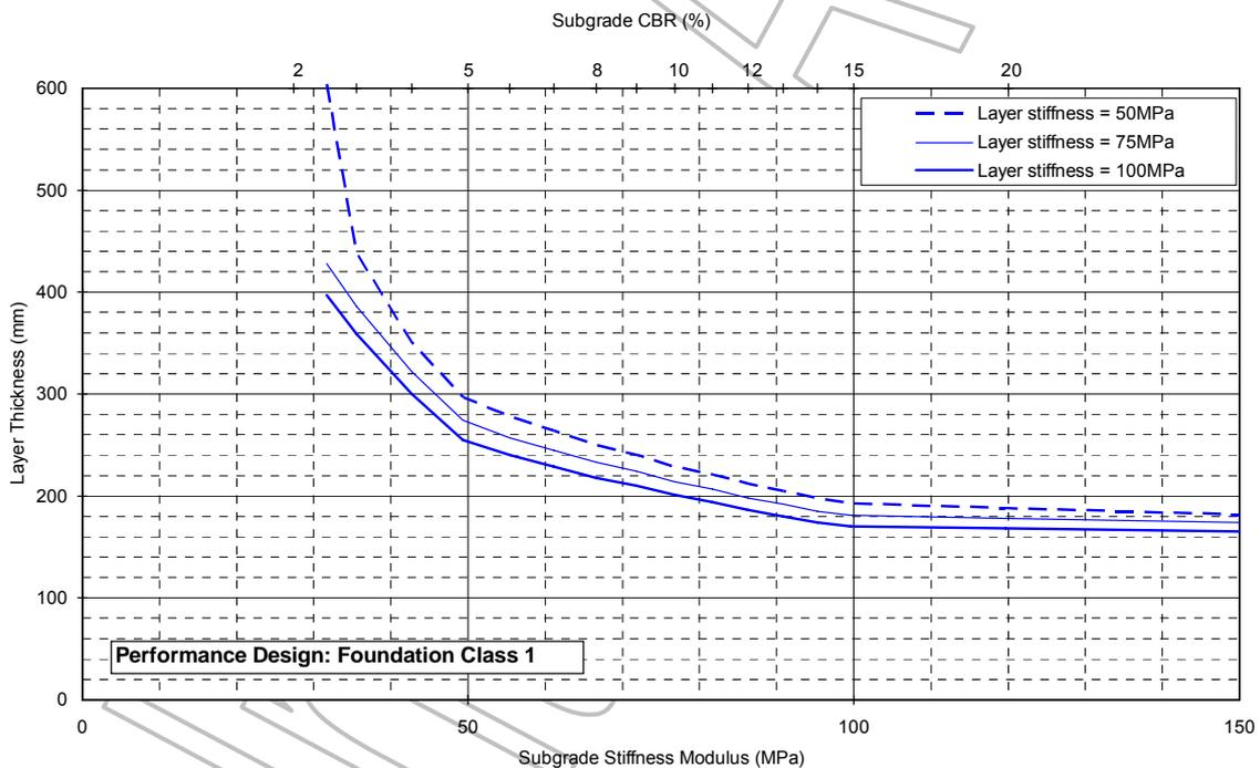
**FIGURE 4.2 Class 1 Designs – Single Foundation Layer**
