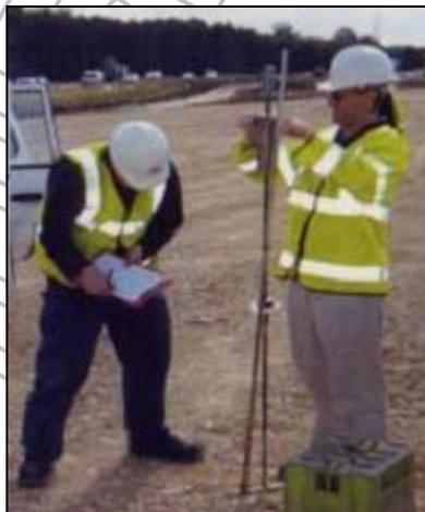
**FIGURE 7.2 The Dynamic Cone Penetrometer**
