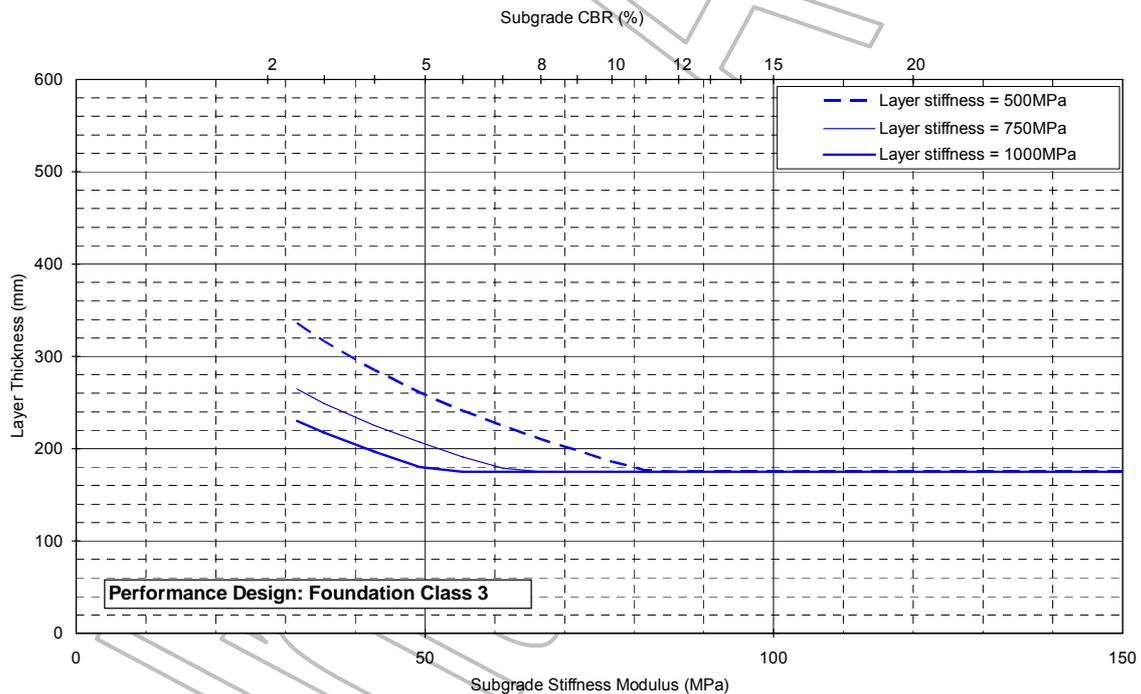
**FIGURE 4.4 Class 3 Designs – Single Foundation Layer**
