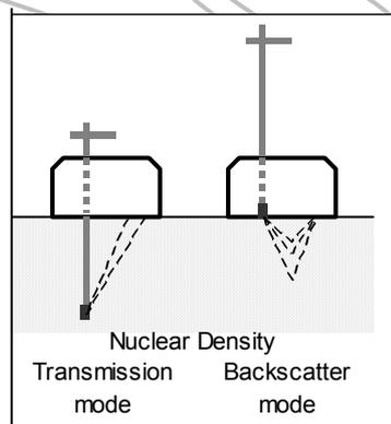
Figure 7.1 Density Testing Apparatus
