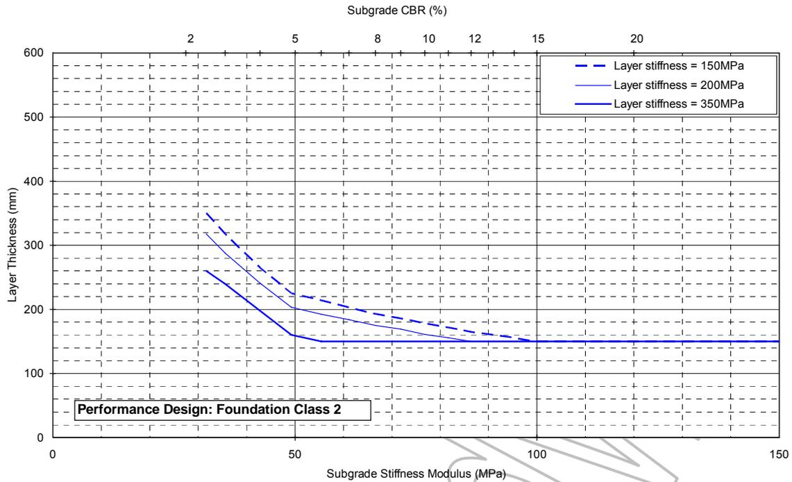
**FIGURE 4.3 Class 2 Designs – Single Foundation Layer**
