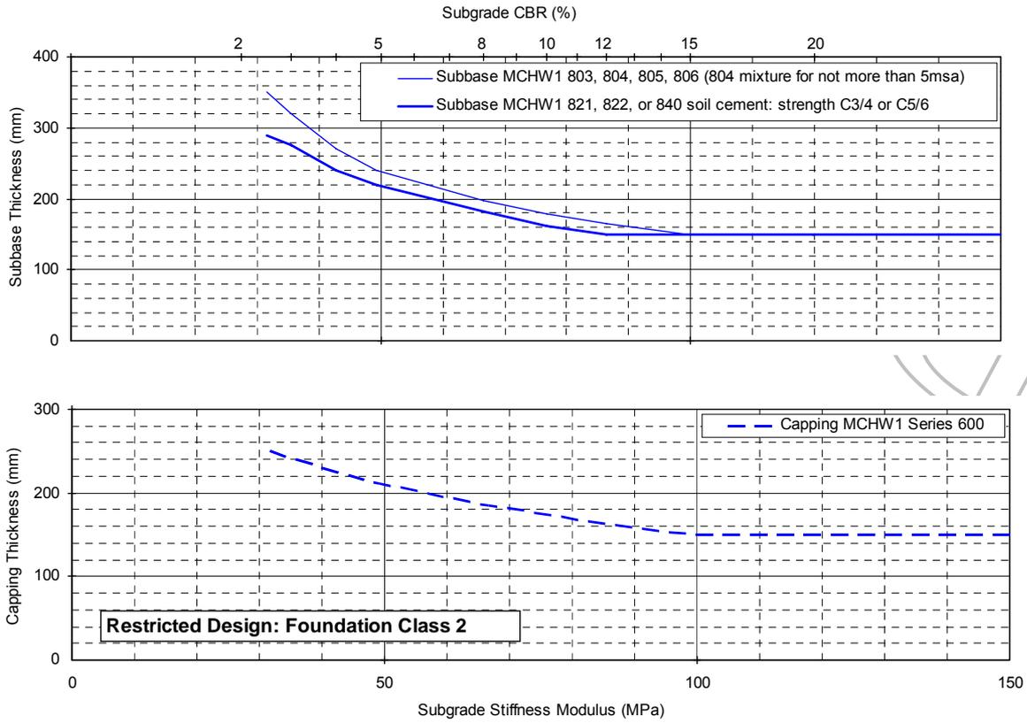
**FIGURE 3.2 Restricted Design Options – Class 2 Subbase on Capping**
