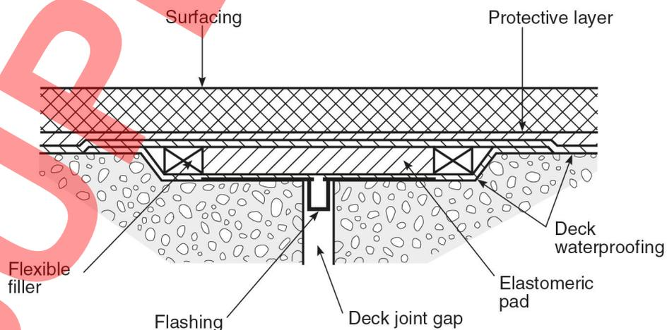
Various materials have been used to form buried joints, such as copper-lined bituminous sheeting, quarry tiles, Formica or similar, or steel plates. These materials have had varying degrees of success depending on the horizontal movements and traffic loads imposed. The principal problem where rigid plates have been used is that they are difficult to bed down properly and subsequent rocking under traffic loading has been a major cause of premature failure of the joint system.
