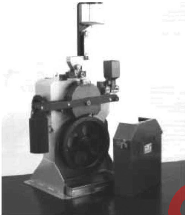
Figure 3.2: Accelerated Polishing Machine
