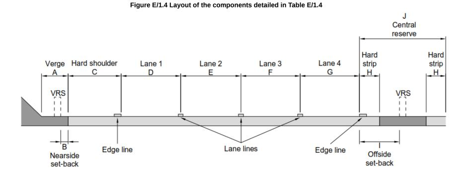
Table E/1.4 Reduced cross-sections hierarchy for widening on existing motorway mainline carriageways
