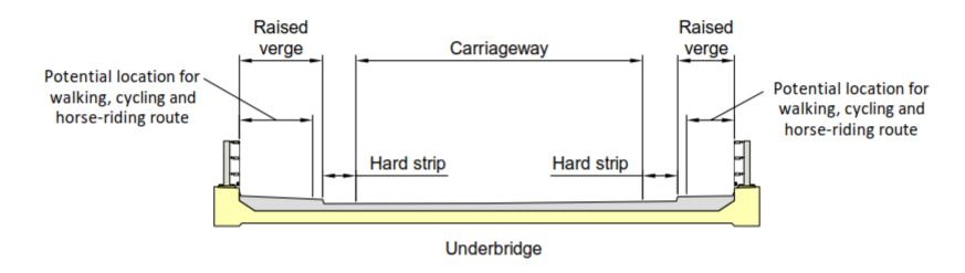
3.1.2 Where it is necessary to divide lanes of a single carriageway at divided structures (see Figure 3.1.2), the carriageway dimensions should be in accordance with those identified for single-lane dualling on single carriageway roads in CD 123 [Ref 11.N].
