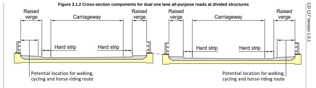
NOTE Occasionally it is necessary to provide a single lane in each direction separated by a central reserve.
