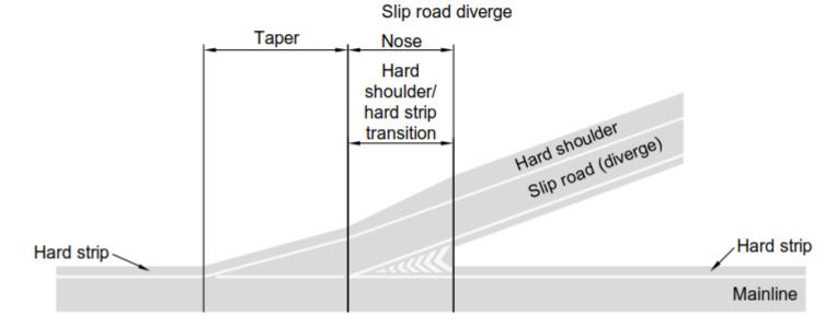
2.30.1 Gain and loss of the offside hard strip on connector roads with superelevation should be as shown in Figure 2.30.1
