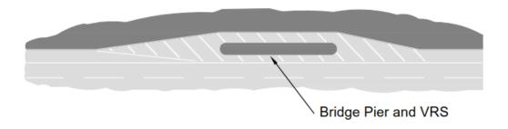
E/1.19 The taper at the start of the hatching in the hard shoulder where an emergency access route is provided behind a bridge pier shall have a ratio of 1:15.
