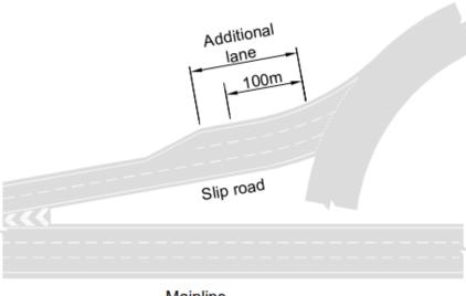
2.19 Where the additional lane(s) extend upstream beyond a point level with the back of diverge nose the additional lane(s) provided shall extend at least as far upstream as the tip of the diverge nose (see Figure 2.19).
