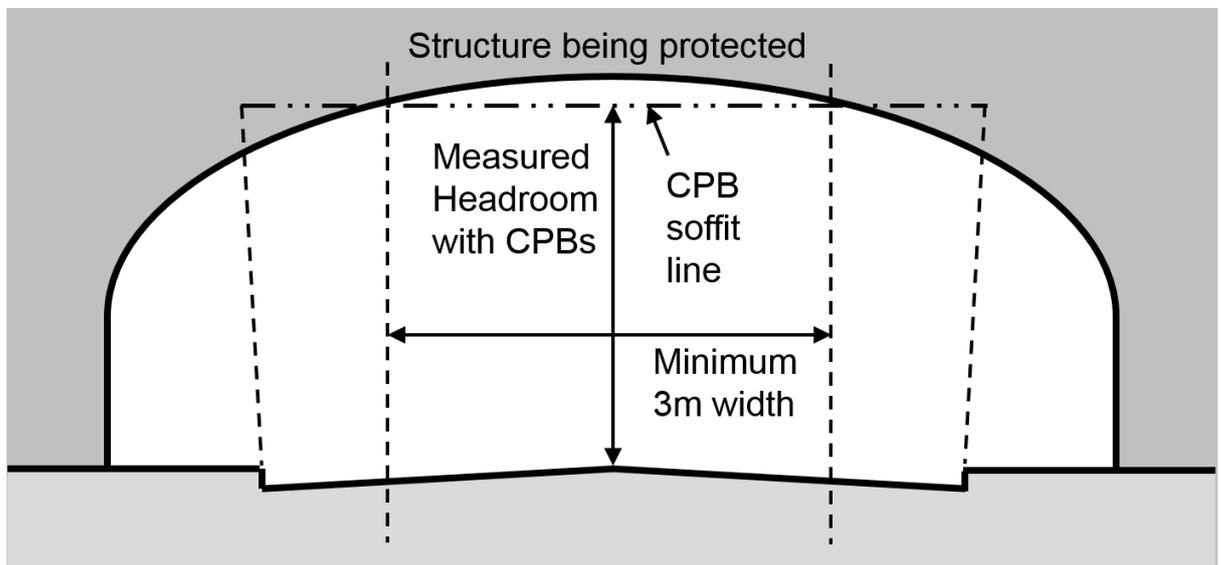
3.12 The CPB shall be pre-cambered where necessary to achieve the desired profile after permanent deflection.
