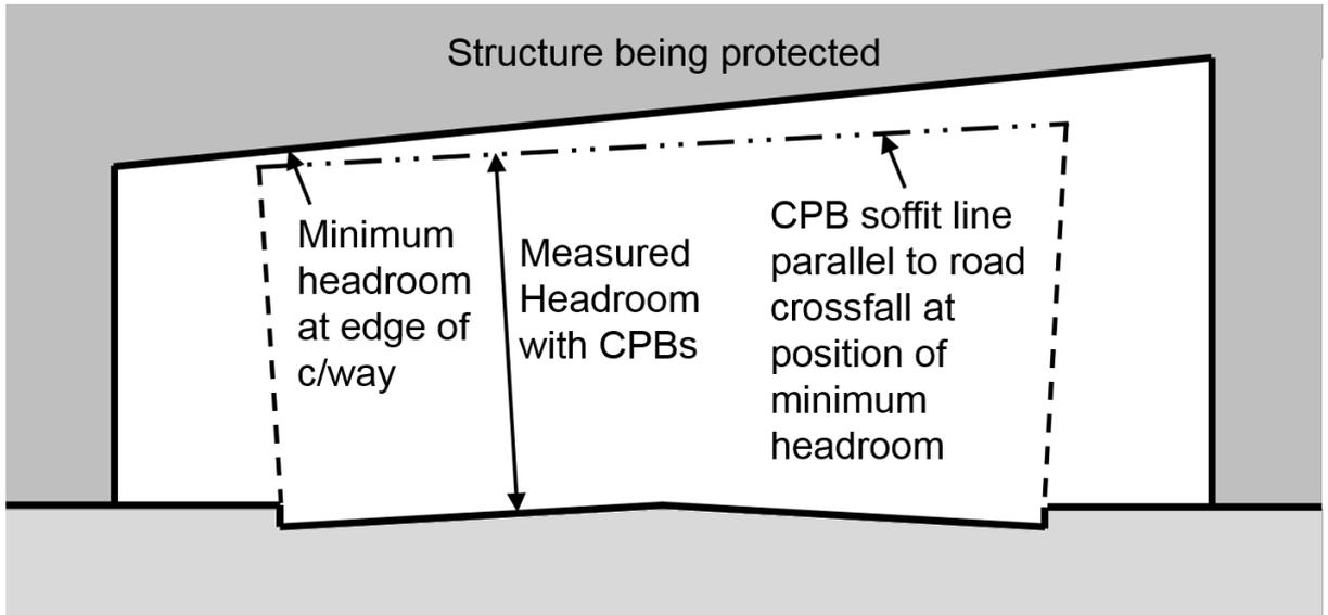
3.11 For arched structures, the CPB levels shall be set to maximise measured headroom over a minimum 3m width of carriageway as shown in Figure 3.11.
