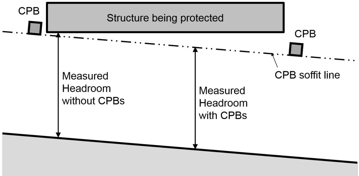
3.9 For non-arched structures where the minimum headroom is at the crown of the carriageway under the bridge, the CPB shall be parallel to the structure soffit, as shown in Figure 3.9.
