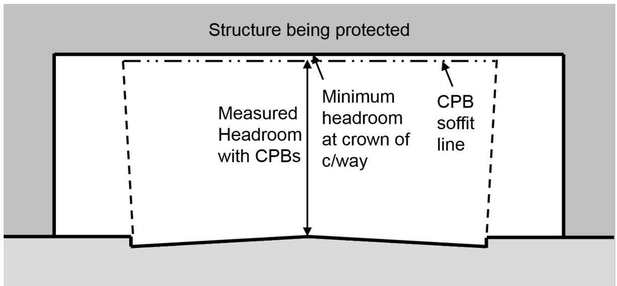
3.10 For non-arched structures where the minimum headroom is at the edge of the carriageway under the bridge, the CPB shall be parallel to the road crossfall at the minimum headroom position, as shown in Figure 3.10.
