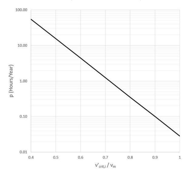
Figure 5.7b Factor for orientation of bridge in plan
