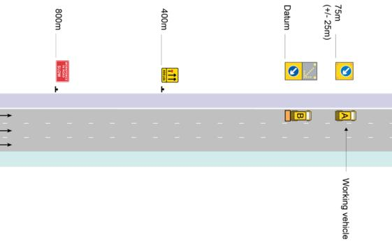
Figure E/2.5 Plan STC 1: Short term closure technique - type 1
