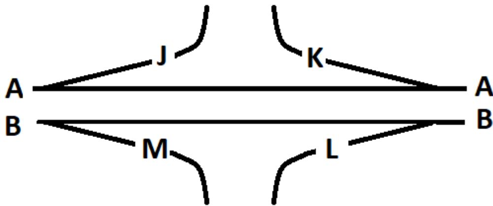
**NOTE** The lettering as shown in Figure E/1.7 is specific to the main carriageway identifiers, i.e. an exit slip from the "A" carriageway is always designated as "J".
