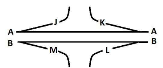
Figure E/1.7 Carriageway identifiers on connector roads
