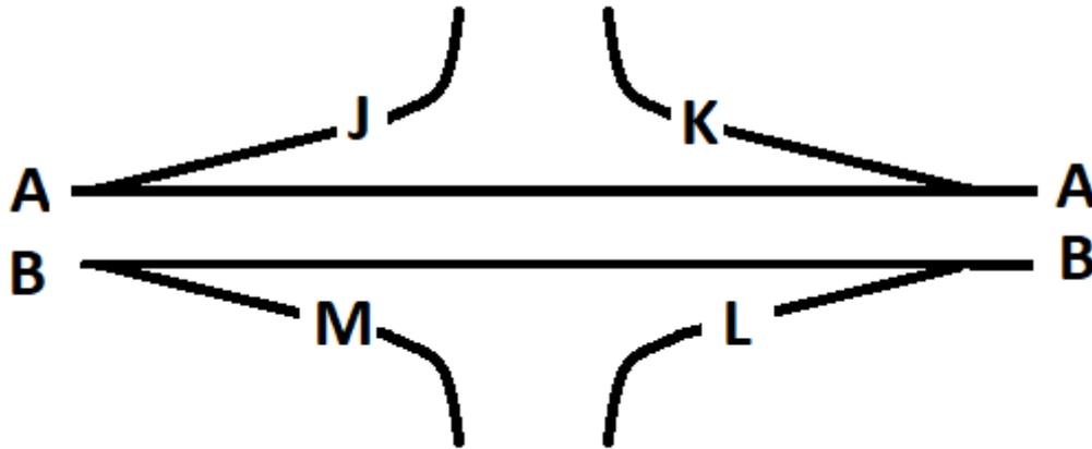
**NOTE** The lettering as shown in Figure E/1.7 is specific to the main carriageway identifiers, i.e. an exit slip from the "A" carriageway is always designated as "J".
