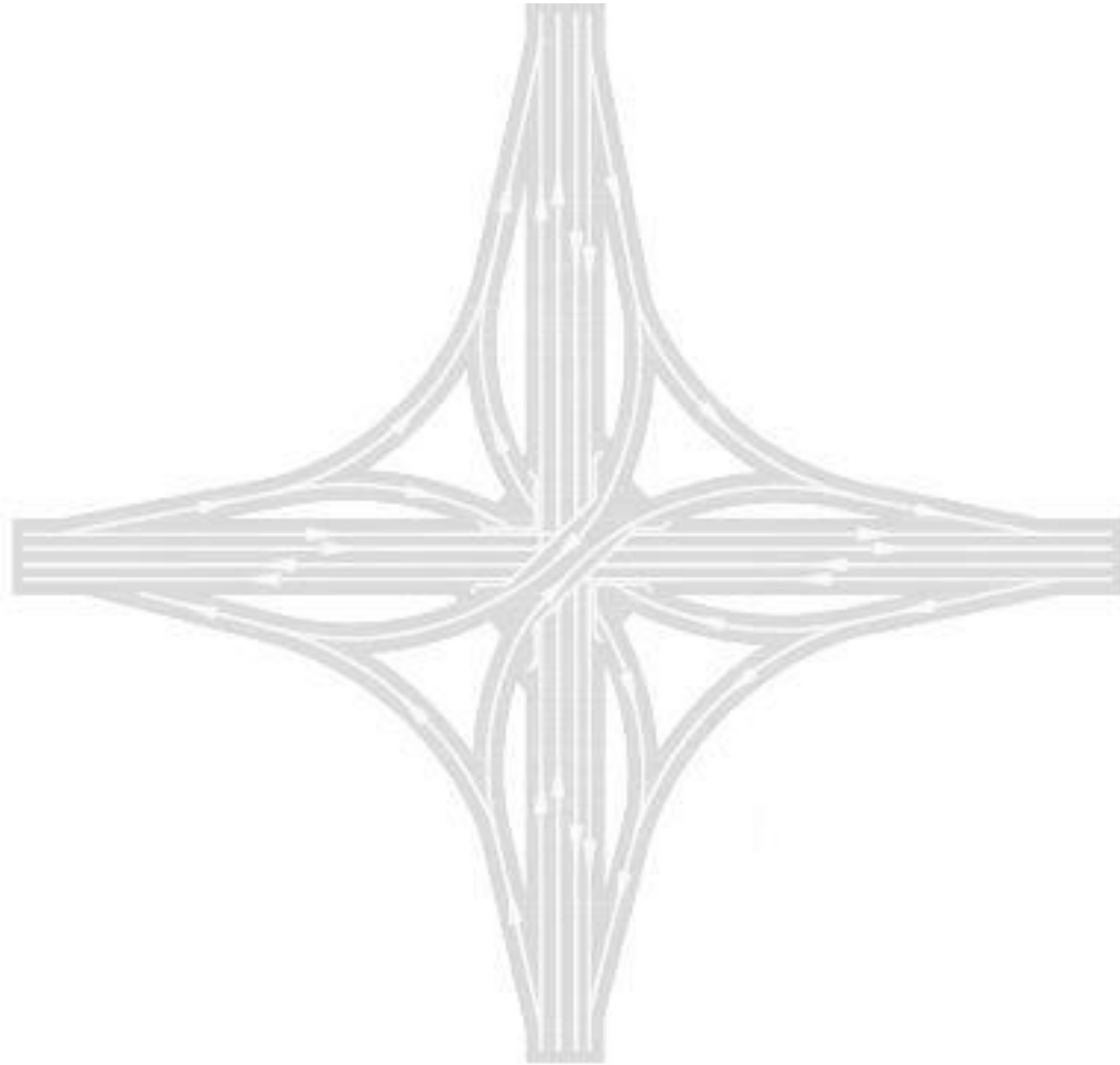
Figure A.9 4-way, 4-level interchange layout
