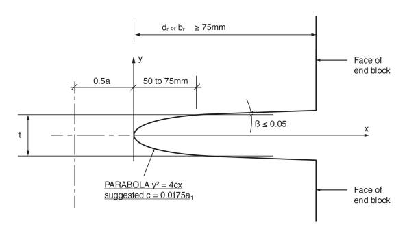
Figure A.2 Typical shape of a parabolic notch
