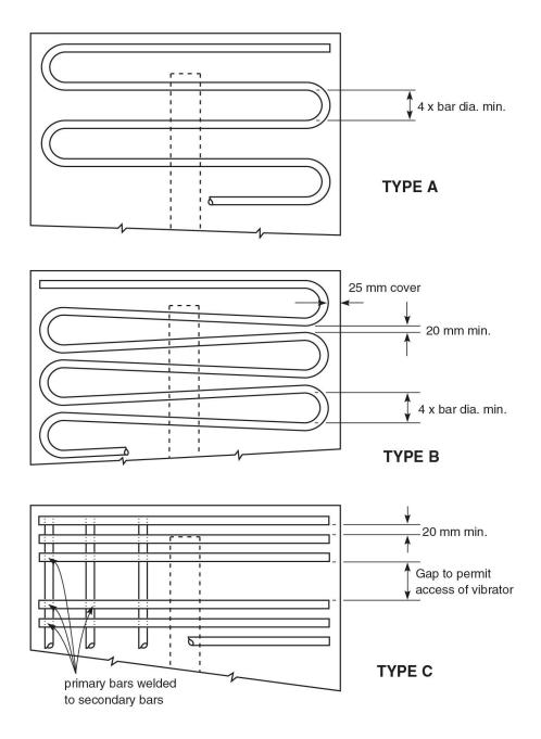
Examples of typical mat reinforcement which were proposed for use on end blocks and their respective capacities.
