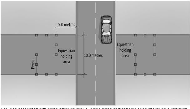
Figure 5.24N3 Equestrian at-grade crossing holding area
