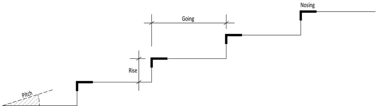
E/4.10.1 The following criteria should be applied to straight and helical stairs:
