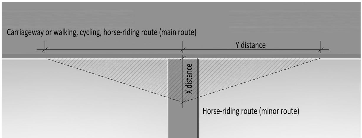
5.6 "Y" distances shall be measured from an eye height of 1.5 metres to 2.7 metres for equestrians.
