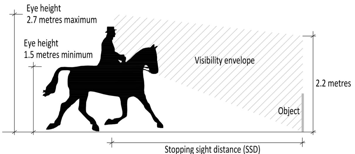
**NOTE** The object height is taken as a range so that equestrians can observe deformations, holes and objects which could interfere with the horse's progress.
