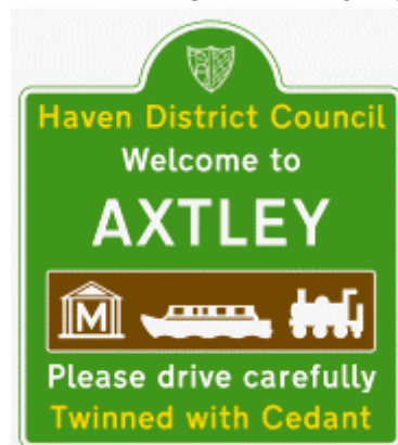
Figure E/4.5N Example of a town or village boundary sign with tourism information
