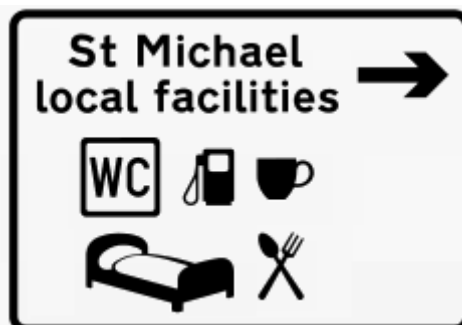
Figure E/6.5N Example of a local facilities sign
